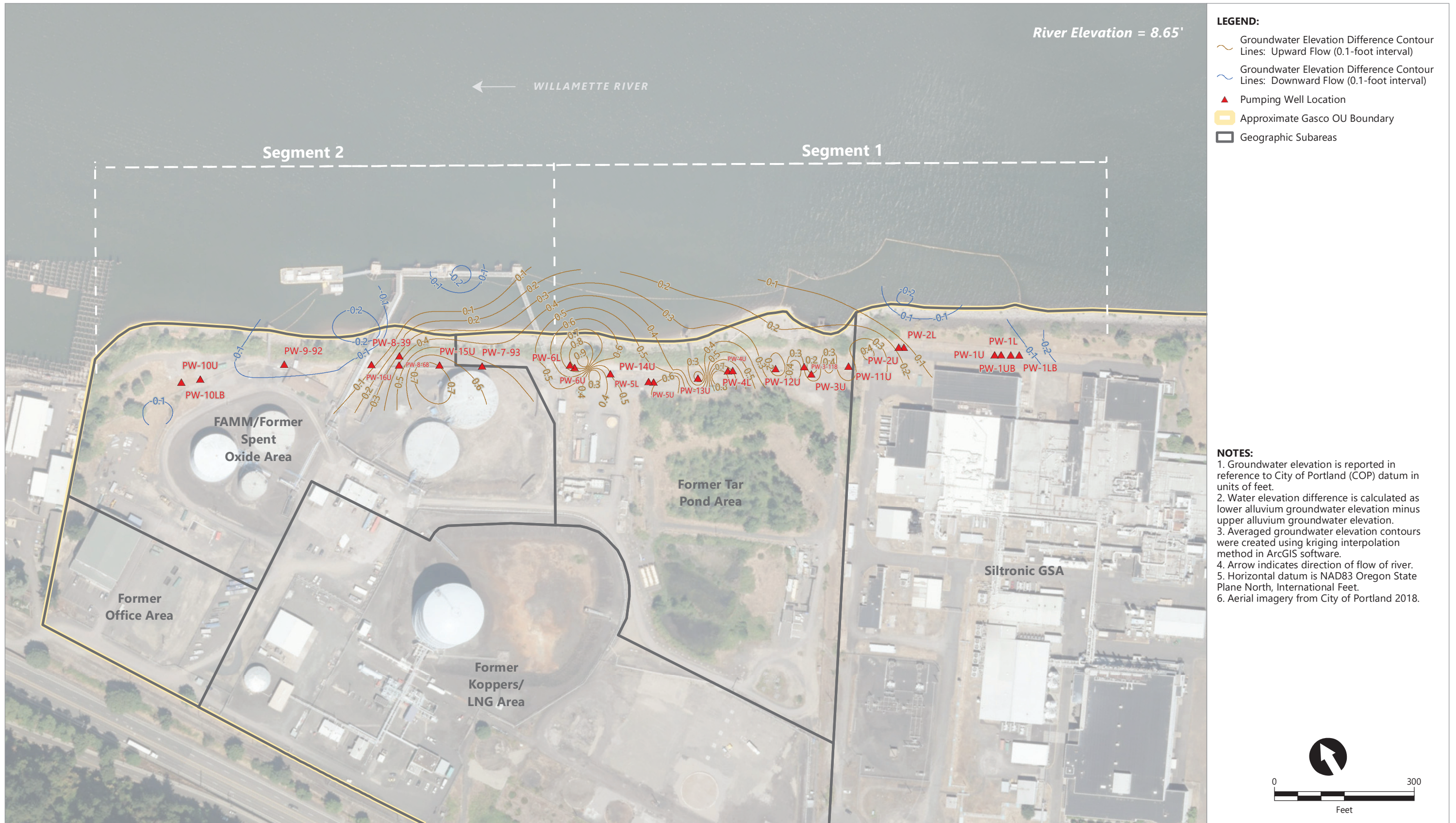
Figure 6.2 Contours of Water Elevation Difference Between Upper and Lower Alluvium Using Serfes 3-Day Rolling Averages From 1/24/2022-1/26/2022
