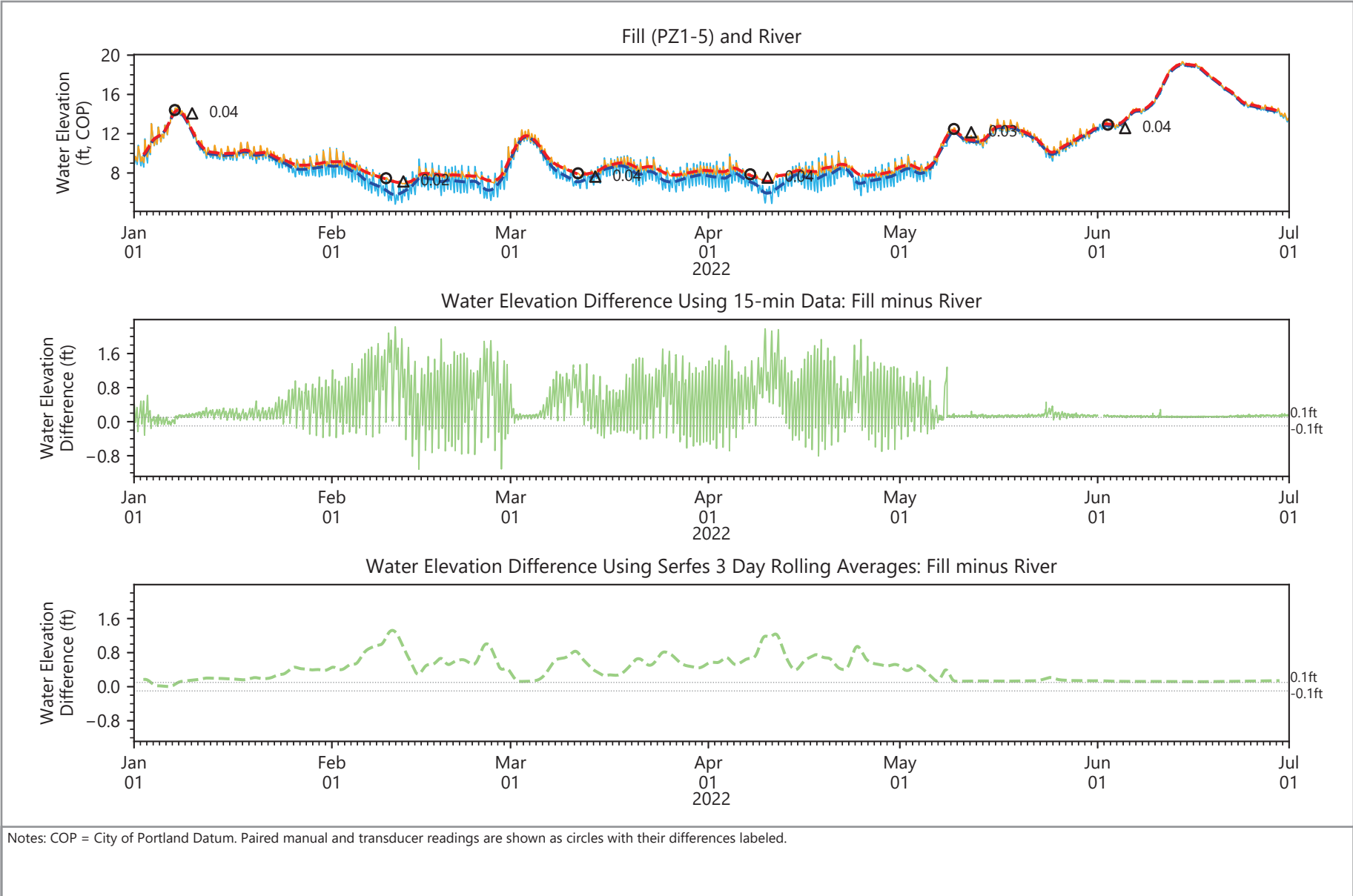
Figure 4.4 Groundwater Elevation Differences NW Natural Gasco Site
