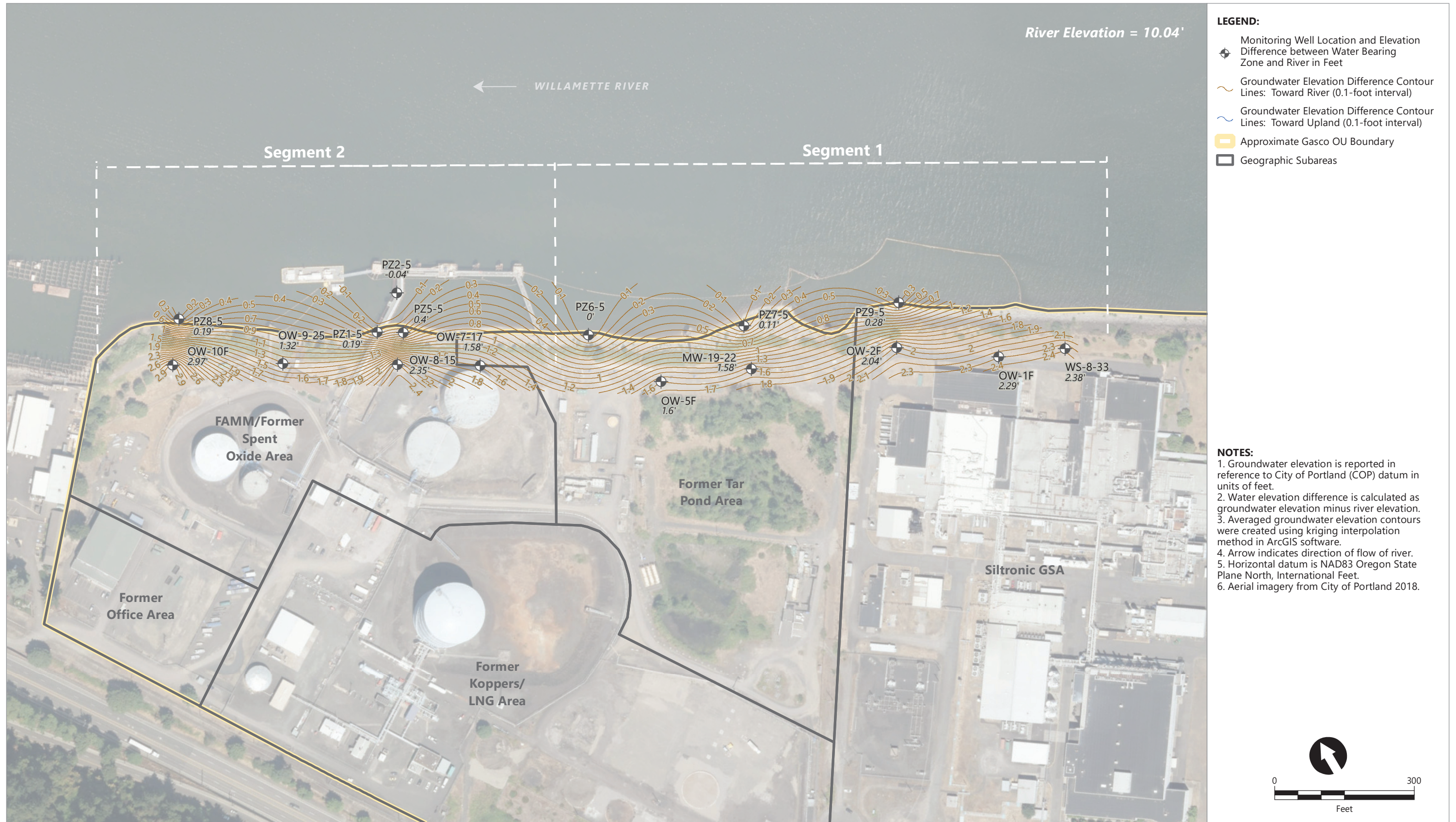
Figure 3.3a Contours of Water Elevation Difference Between Fill and River Using Serfes 3-Day Rolling Averages From 1/11/2022-1/13/2022
