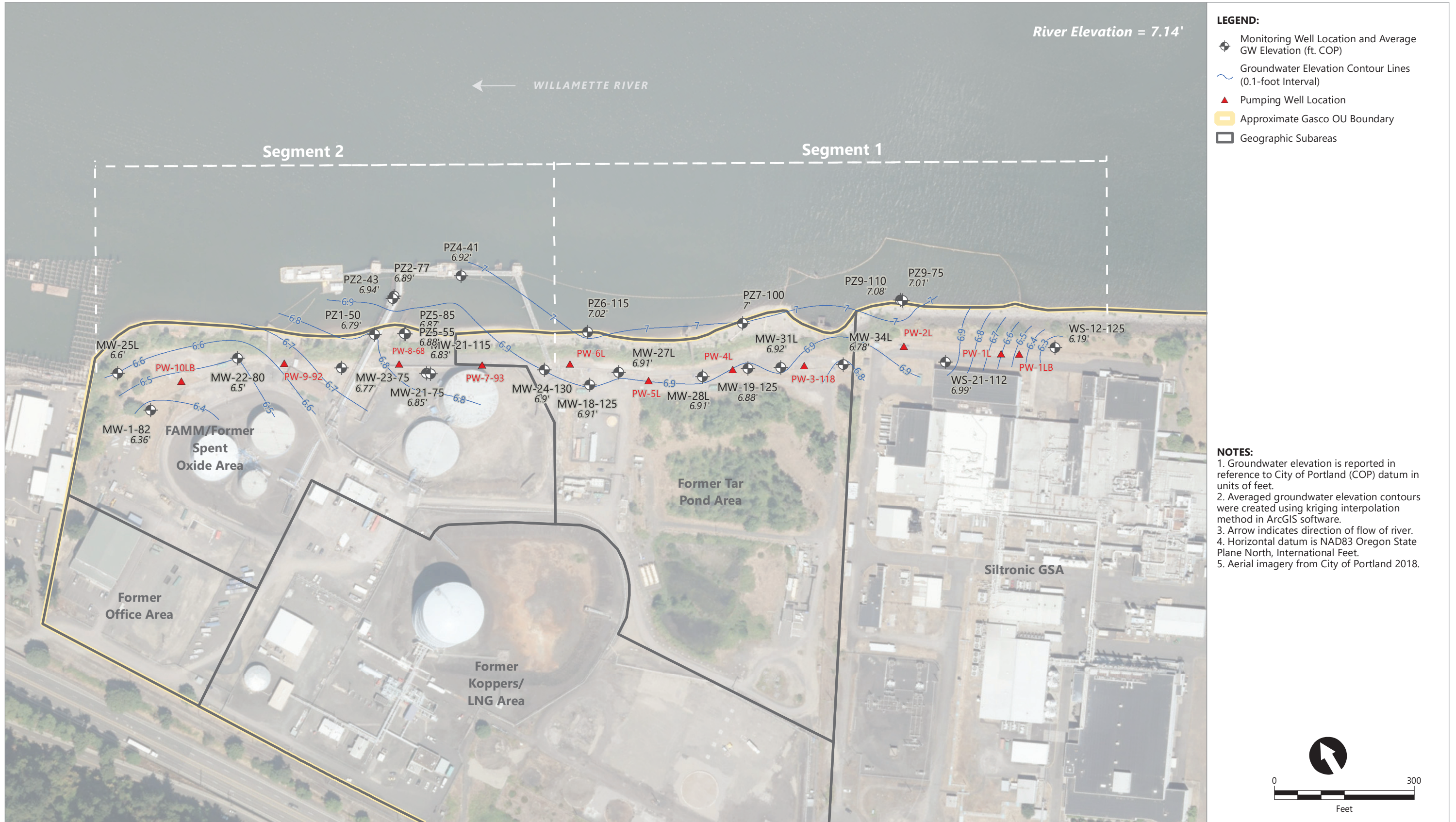
Figure 3.2c Lower Alluvium WBZ Potentiometric Surface Contours Using Serfes 3-Day Rolling Averages From 3/24/2022-3/26/2022
