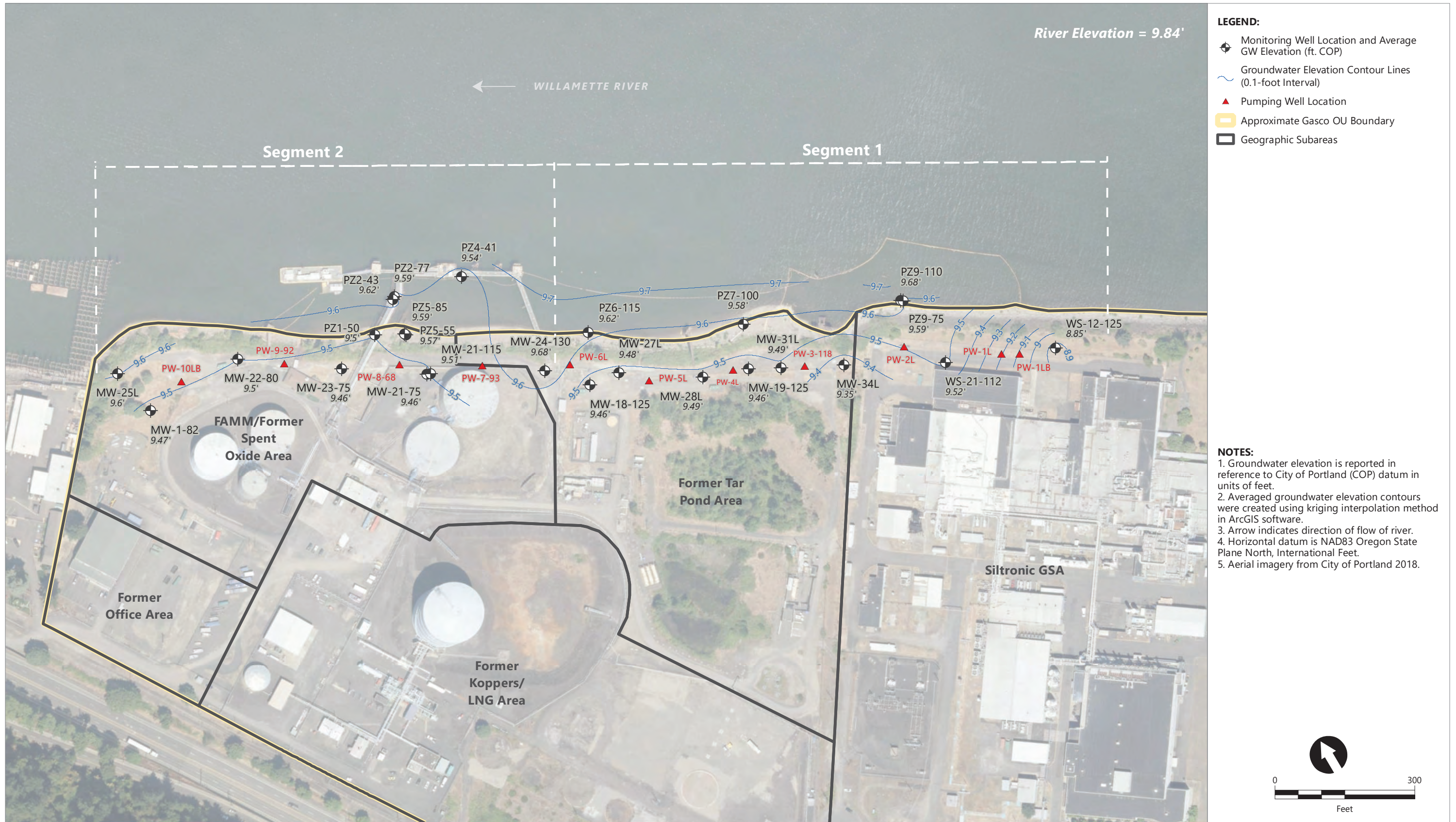
Figure 3.1c Lower Alluvium WBZ Potentiometric Surface Contours Using Serfes 3-Day Rolling Averages From 7/11/2022-7/13/2022
