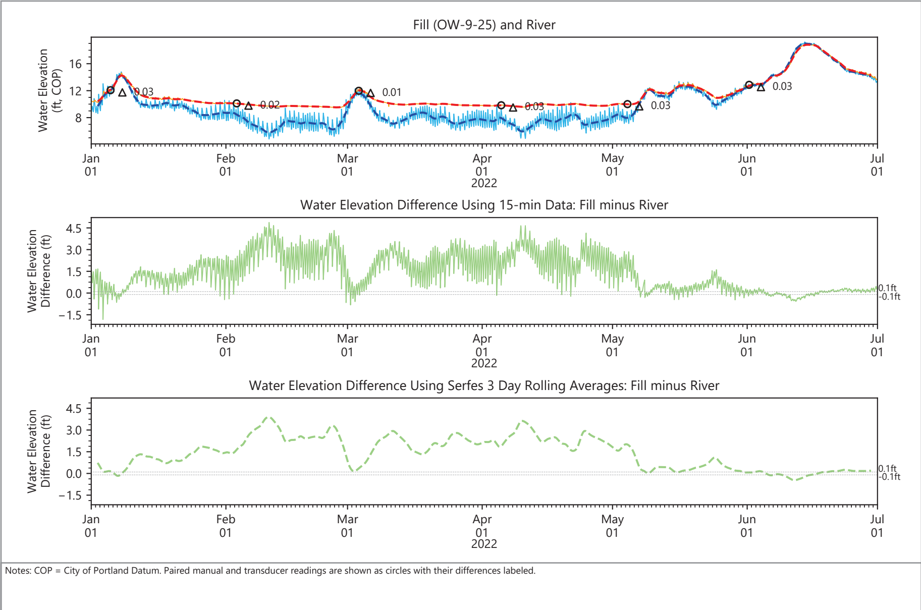
Figure 4.3 Groundwater Elevation Differences NW Natural Gasco Site
