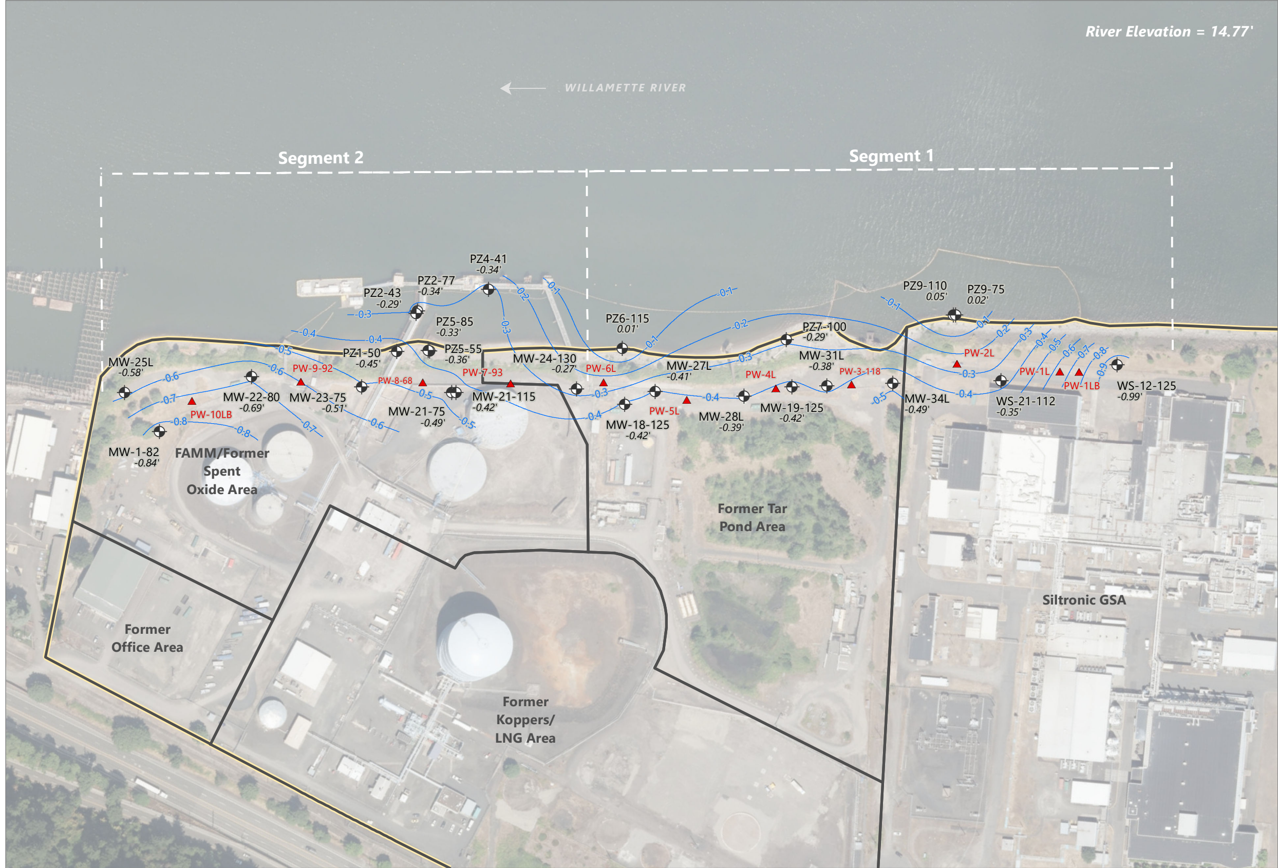
Figure 3.4c Contours of Water Elevation Difference Between Lower Alluvium and River Using Serfes 3-Day Rolling Averages From 6/24/2022-6/26/2022
