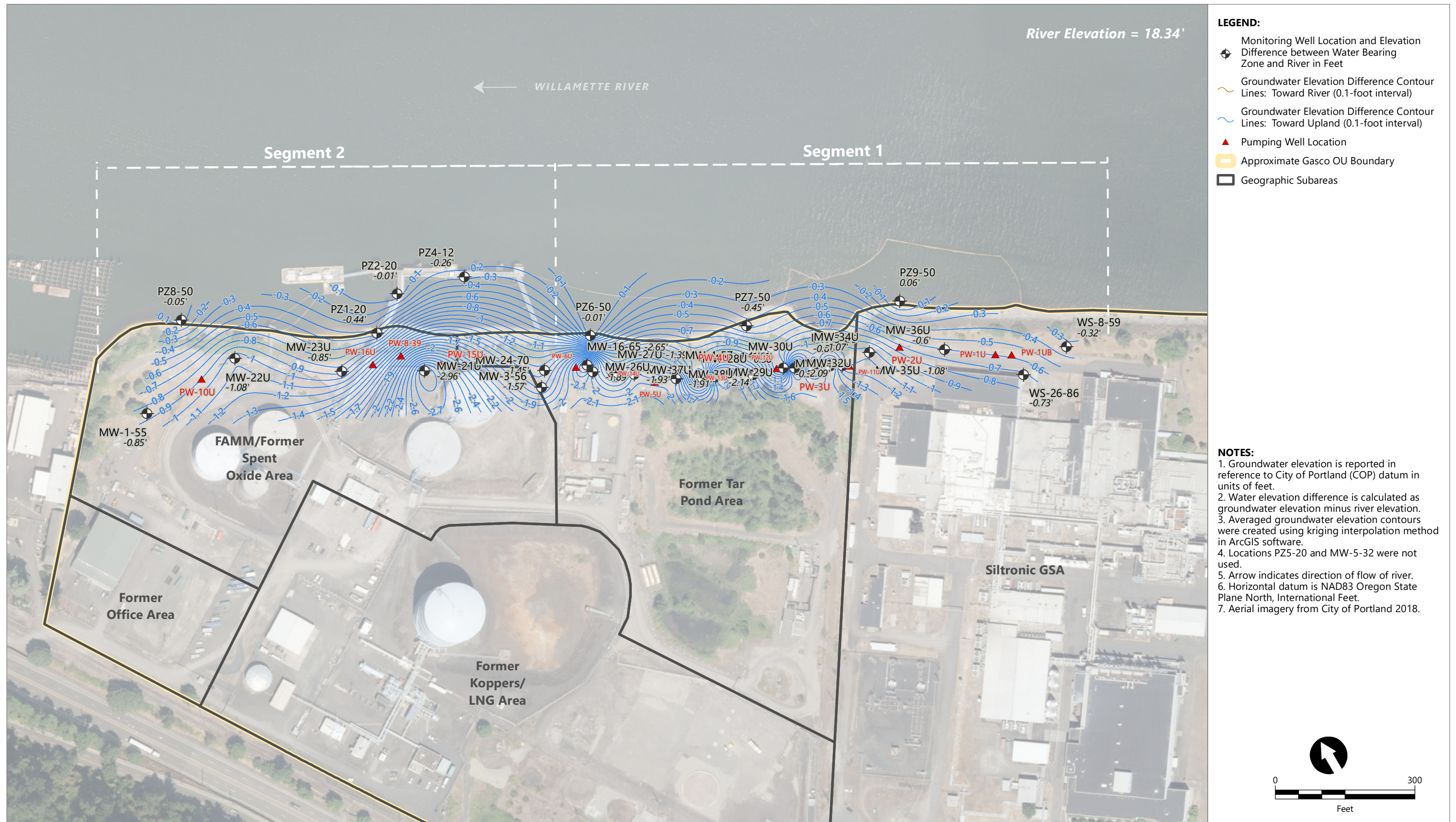
Figure 3.3b Contours of Water Elevation Difference Between Upper Alluvium and River Using Serfes 3-Day Rolling Averages From 6/11/2022-6/13/2022
