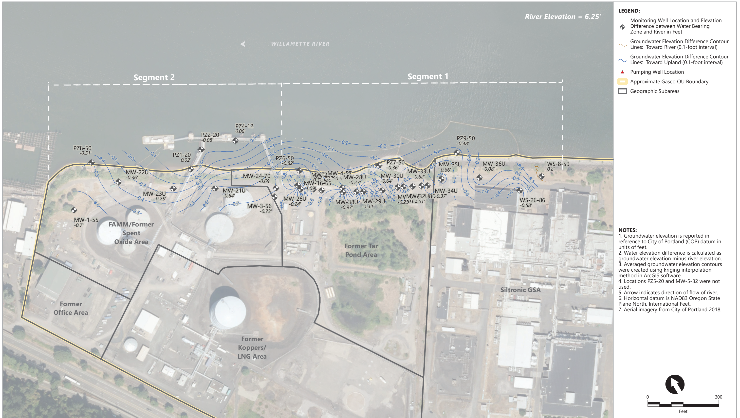
Figure 3.4b Contours of Water Elevation Difference Between Upper Alluvium and River Using Serfes 3-Day Rolling Averages From 2/24/2022-2/26/2022
