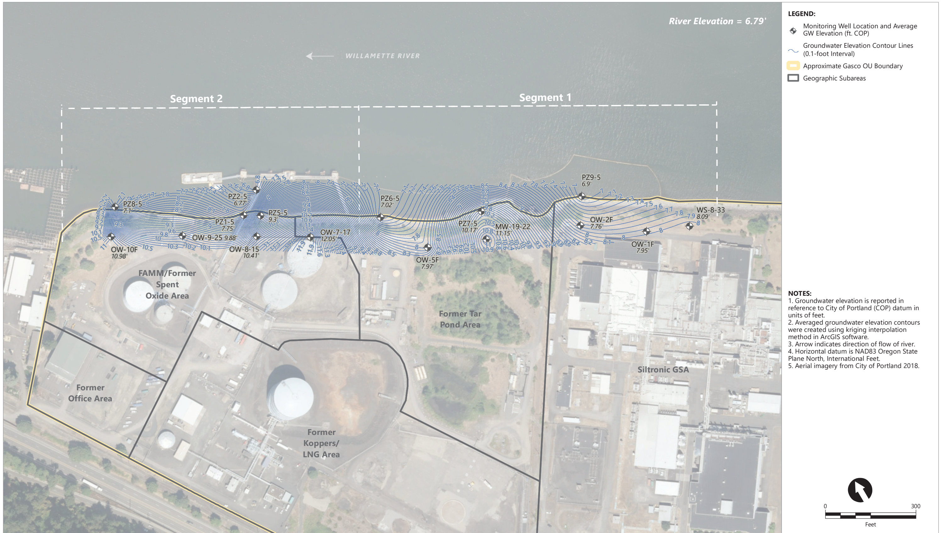
Figure 3.1a Fill WBZ Potentiometric Surface Contours Using Serfes 3-Day Rolling Averages From 4/11/2022-4/13/2022
