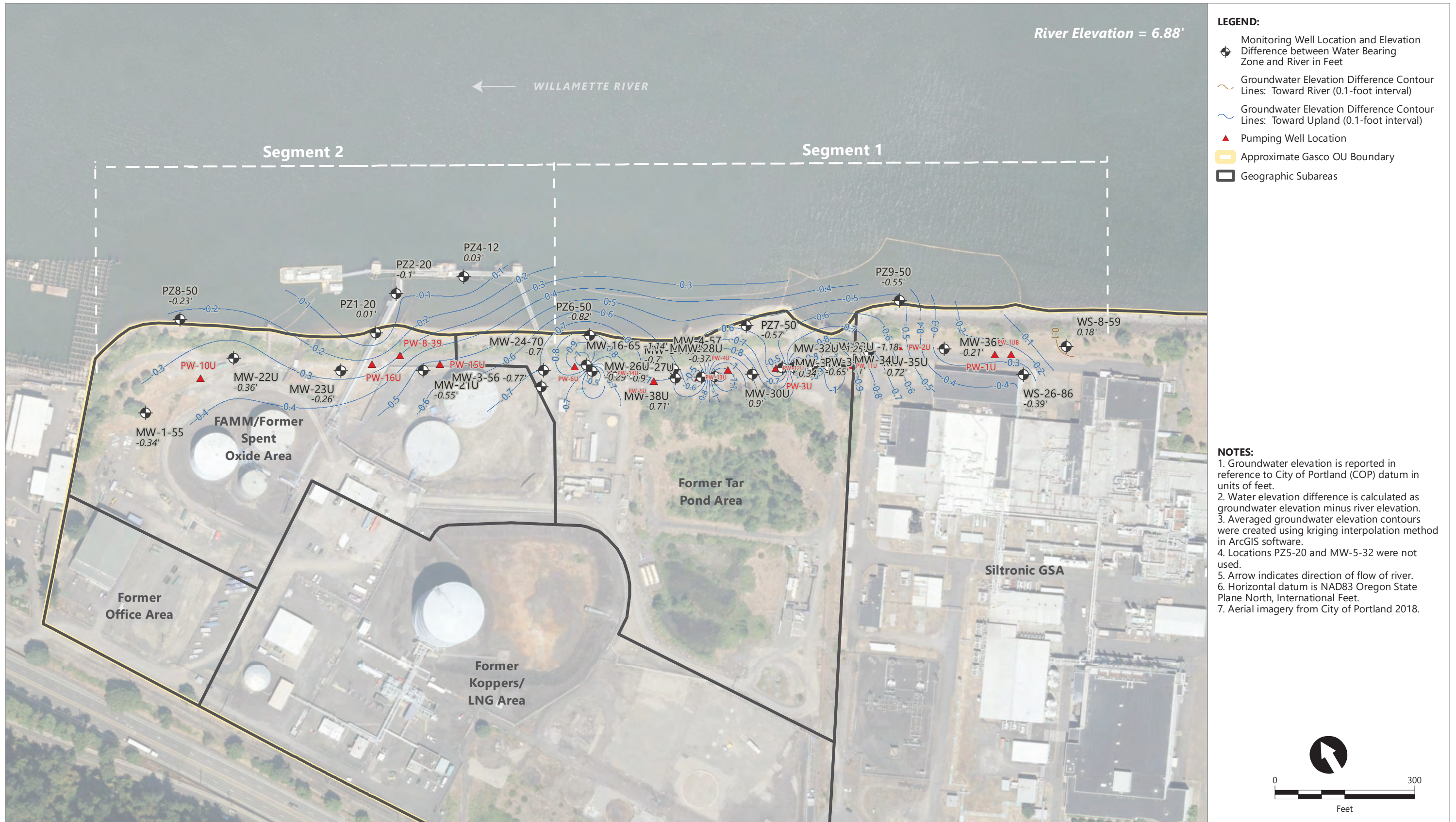
Figure 3.4b Contours of Water Elevation Difference Between Upper Alluvium and River Using Serfes 3-Day Rolling Averages From 7/24/2022-7/26/2022
