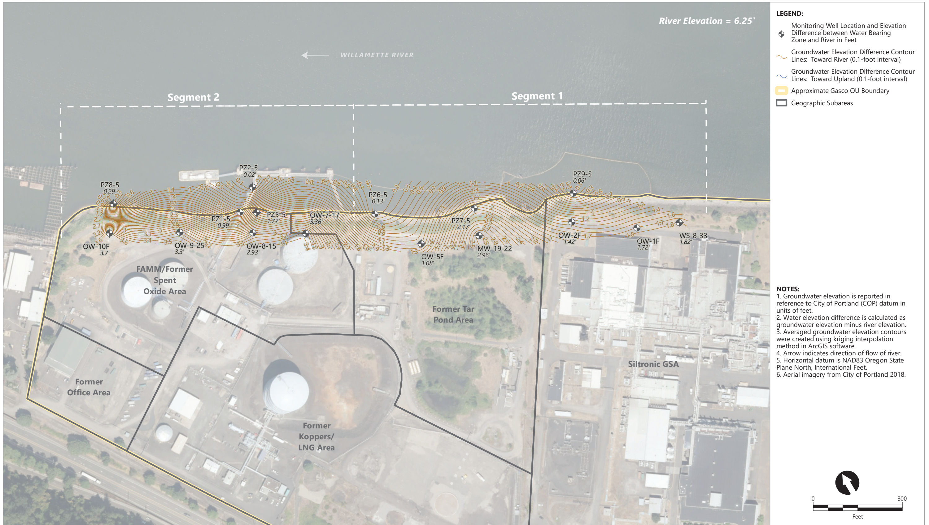
Figure 3.4a Contours of Water Elevation Difference Between Fill and River Using Serfes 3-Day Rolling Averages From 2/24/2022-2/26/2022
