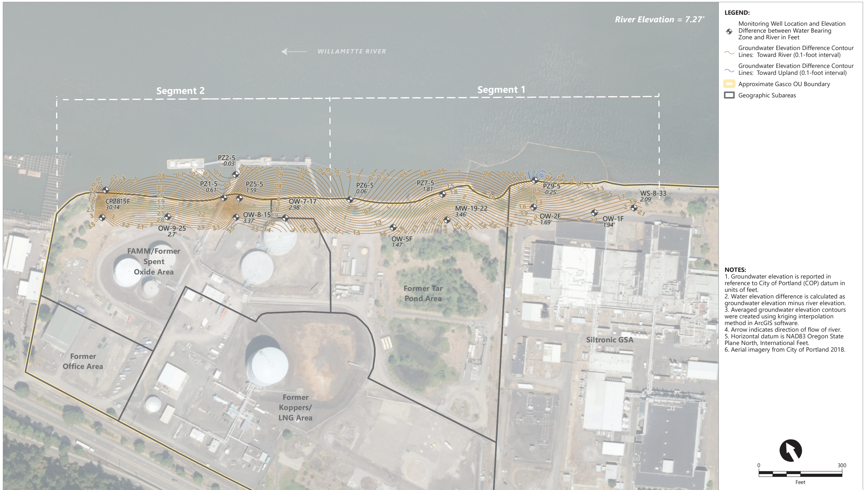
Figure 3.3a Contours of Water Elevation Difference Between Fill and River Using Serfes 3-Day Rolling Averages From 3/11/2022-3/13/2022
