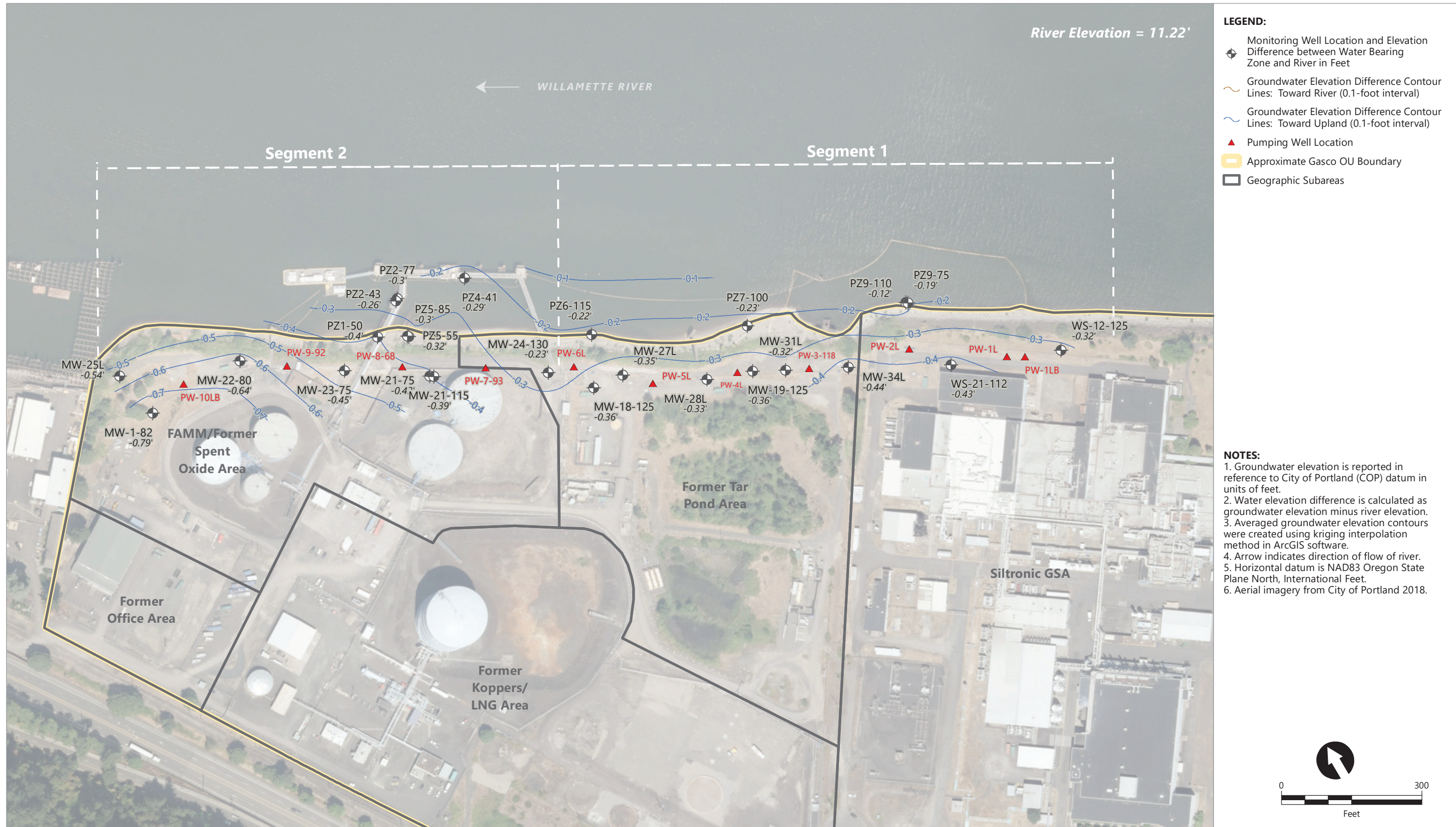
Figure 3.3c Contours of Water Elevation Difference Between Lower Alluvium and River Using Serfes 3-Day Rolling Averages From 5/11/2022-5/13/2022
