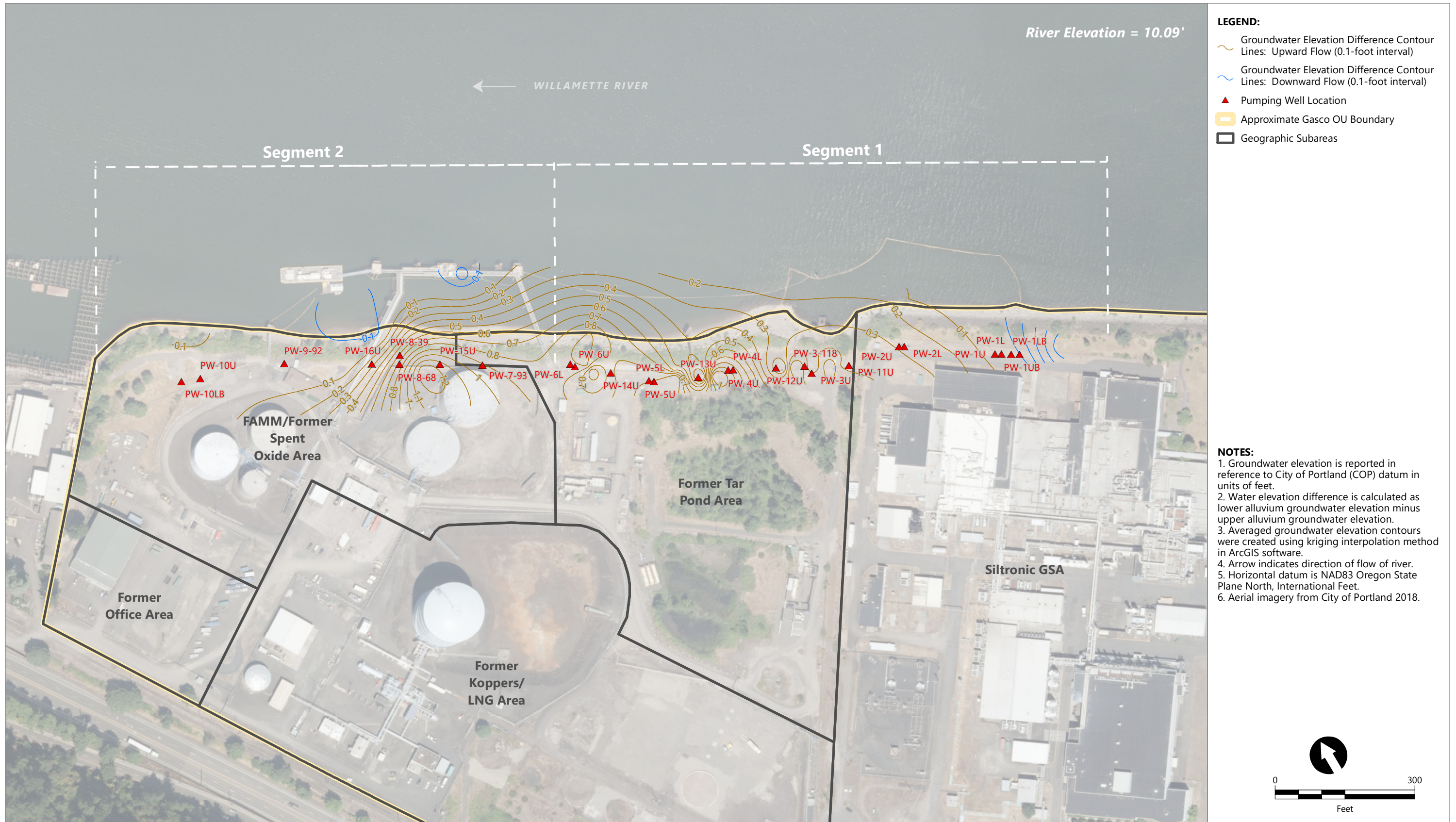
Figure 6.2 Contours of Water Elevation Difference Between Upper and Lower Alluvium Using Serfes 3-Day Rolling Averages From 5/24/2022-5/26/2022
