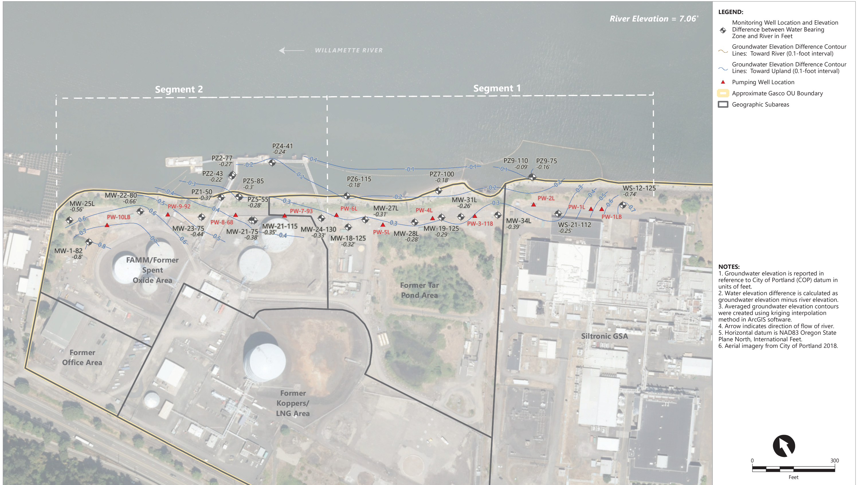
Figure 3.4c Contours of Water Elevation Difference Between Lower Alluvium and River Using Serfes 3-Day Rolling Averages From 4/24/2022-4/26/2022
