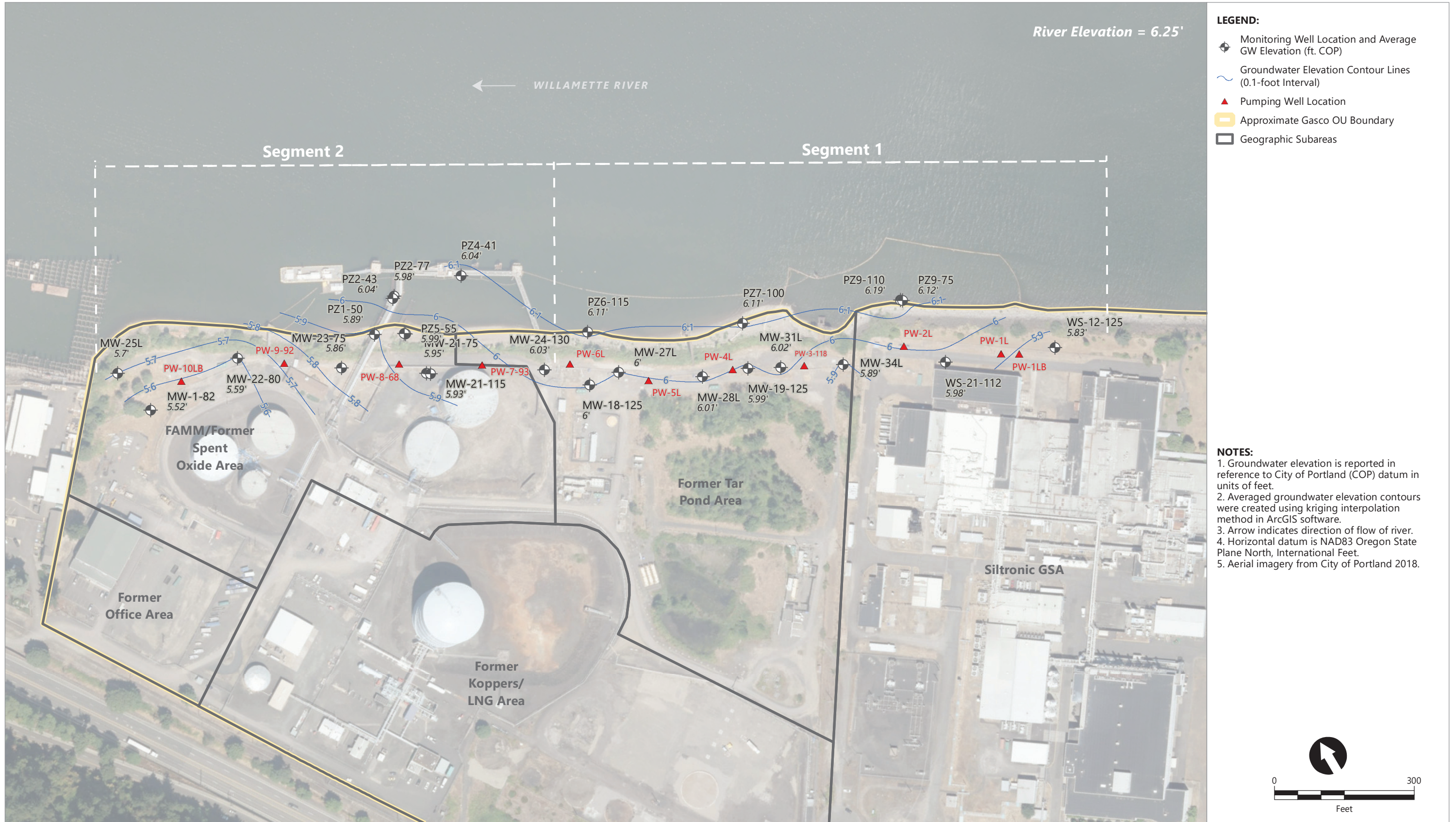
Figure 3.2c Lower Alluvium WBZ Potentiometric Surface Contours Using Serfes 3-Day Rolling Averages From 2/24/2022-2/26/2022
