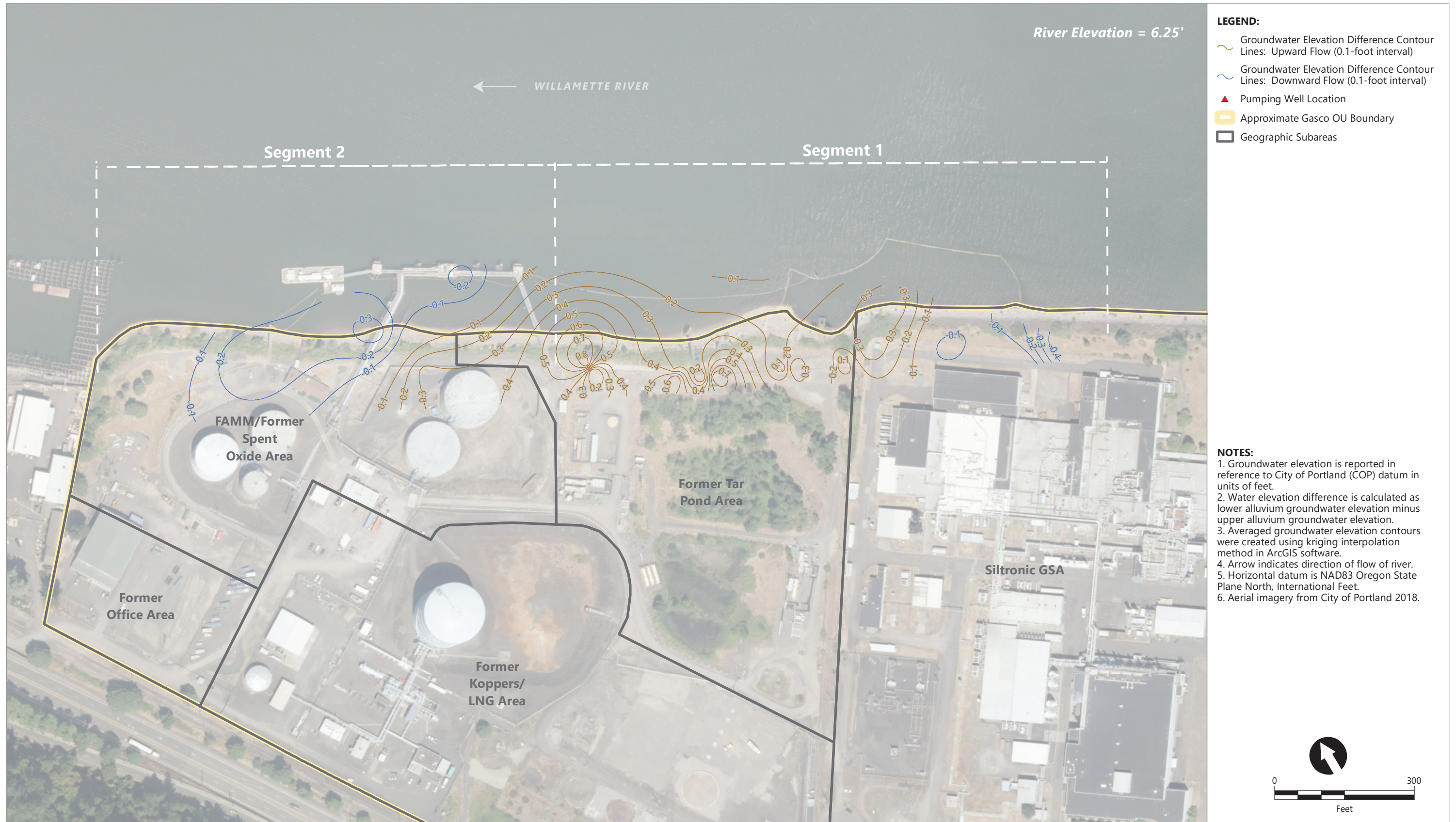
Figure 6.2 Contours of Water Elevation Difference Between Upper and Lower Alluvium Using Serfes 3-Day Rolling Averages From 2/24/2022-2/26/2022
