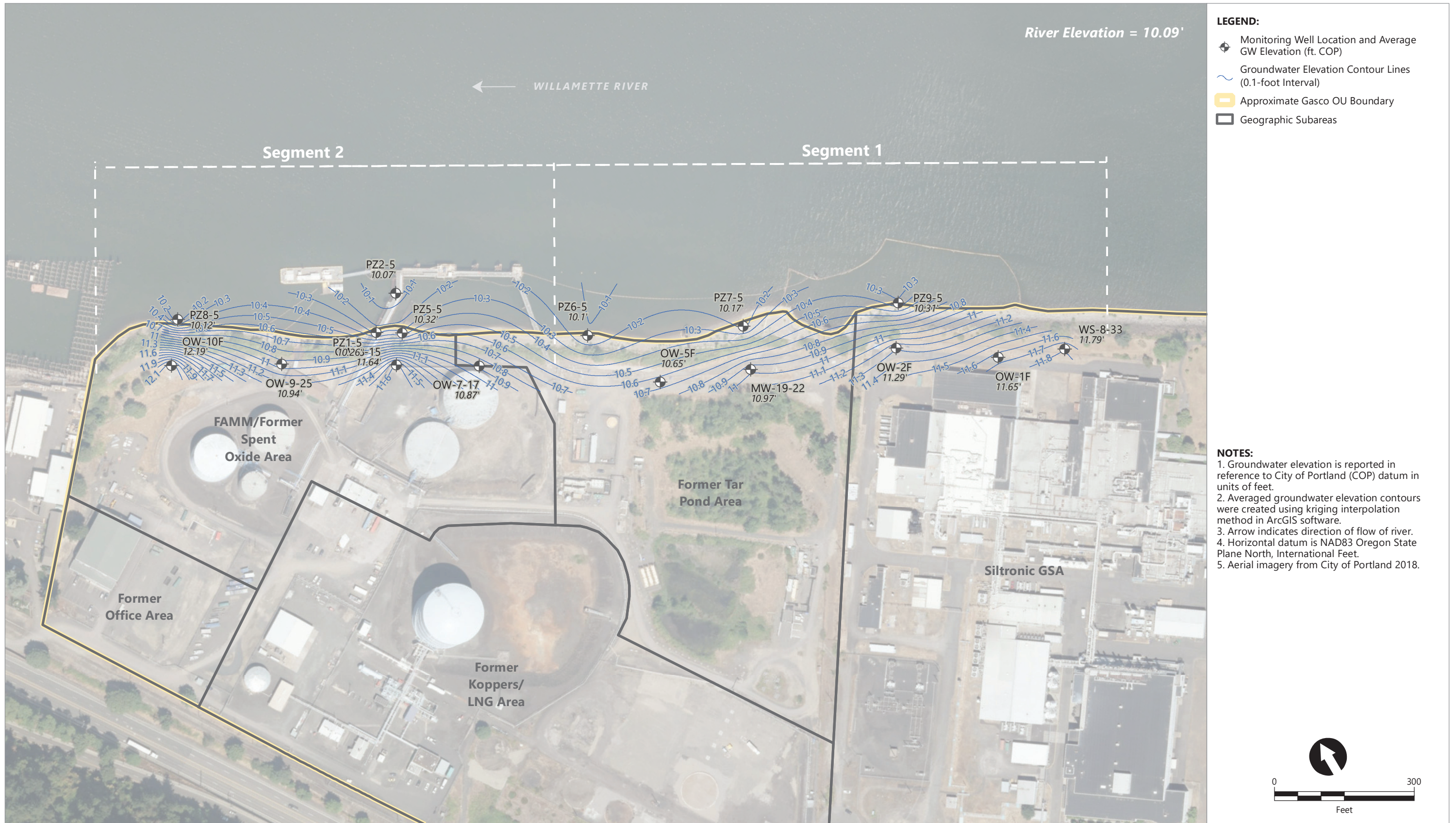
Figure 3.2a Fill WBZ Potentiometric Surface Contours Using Serfes 3-Day Rolling Averages From 5/24/2022-5/26/2022 NWN Gasco Site Portland, Oregon
