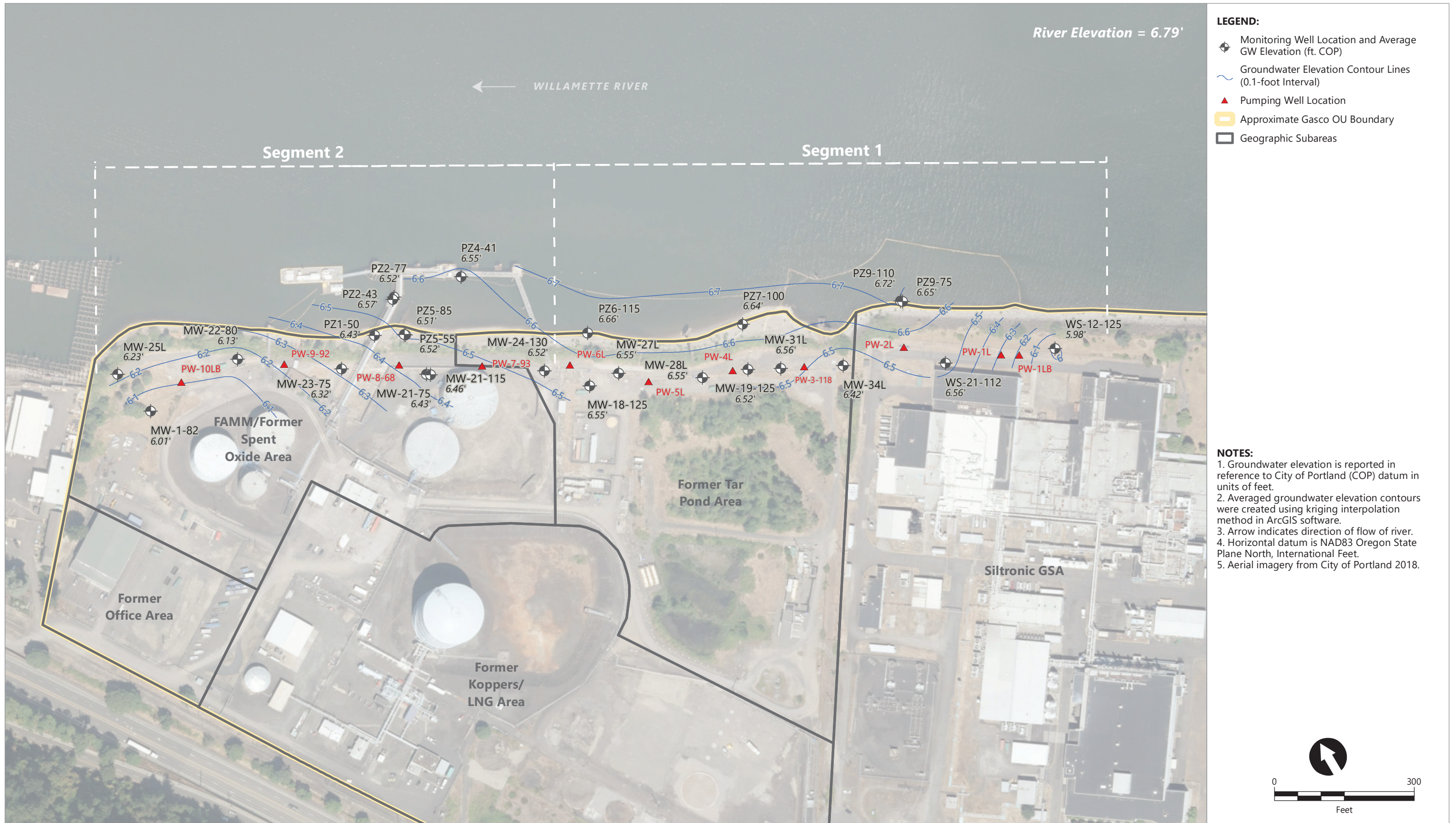
Figure 3.1c Lower Alluvium WBZ Potentiometric Surface Contours Using Serfes 3-Day Rolling Averages From 4/11/2022-4/13/2022
