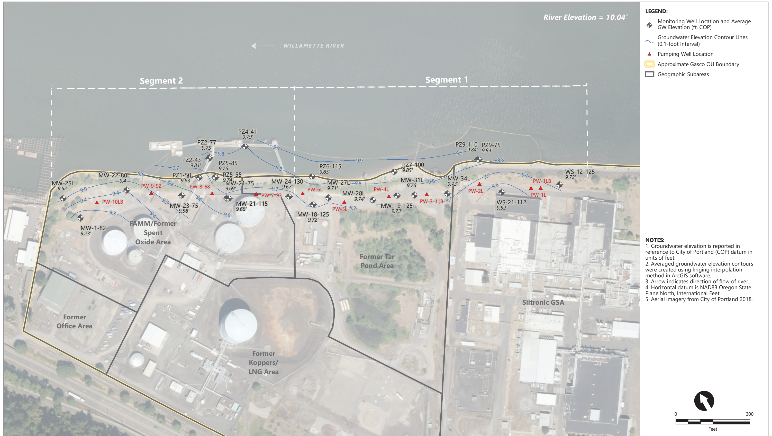
Figure 3.1c Lower Alluvium WBZ Potentiometric Surface Contours Using Serfes 3-Day Rolling Averages From 1/11/2022-1/13/2022
