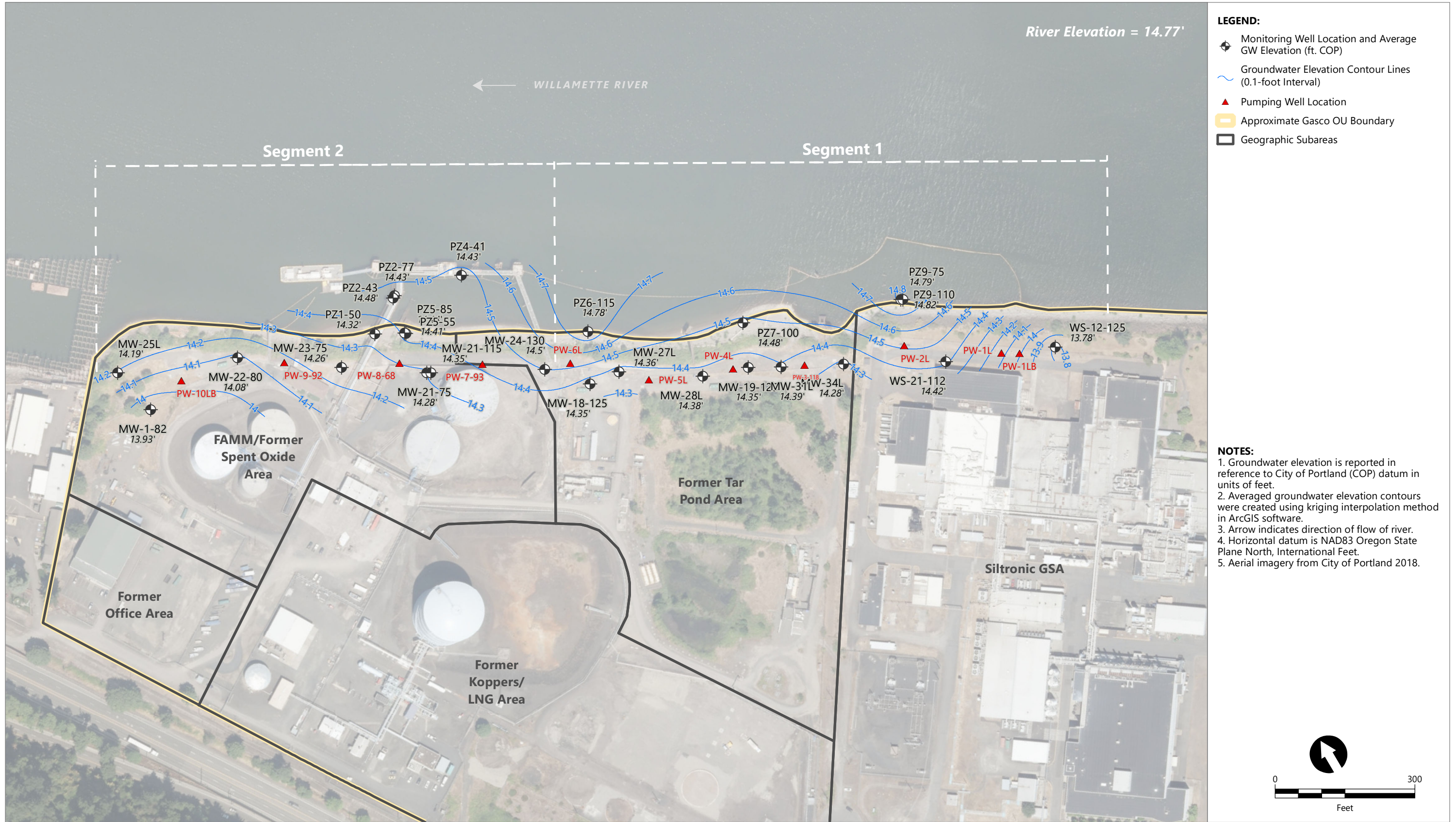
Figure 3.2c Lower Alluvium WBZ Potentiometric Surface Contours Using Serfes 3-Day Rolling Averages From 6/24/2022-6/26/2022
