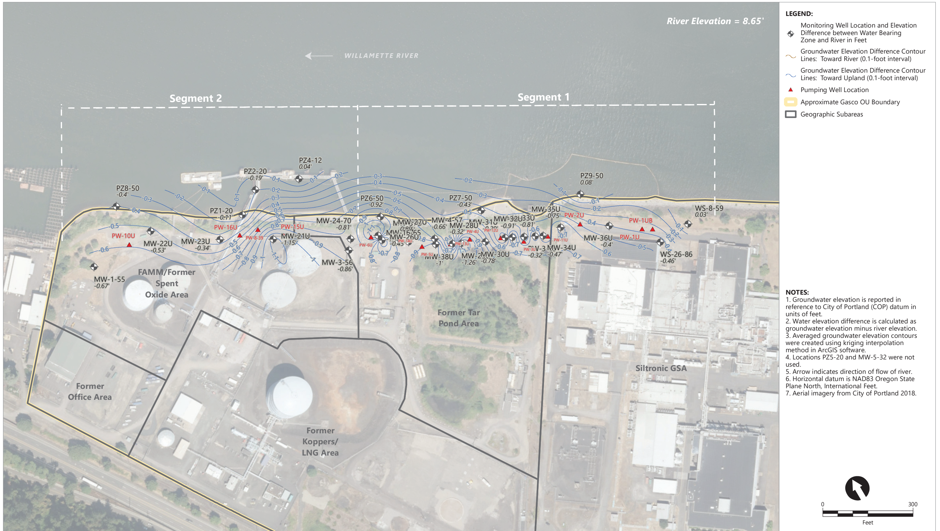
Figure 3.4b Contours of Water Elevation Difference Between Upper Alluvium and River Using Serfes 3-Day Rolling Averages From 1/24/2022-1/26/2022
