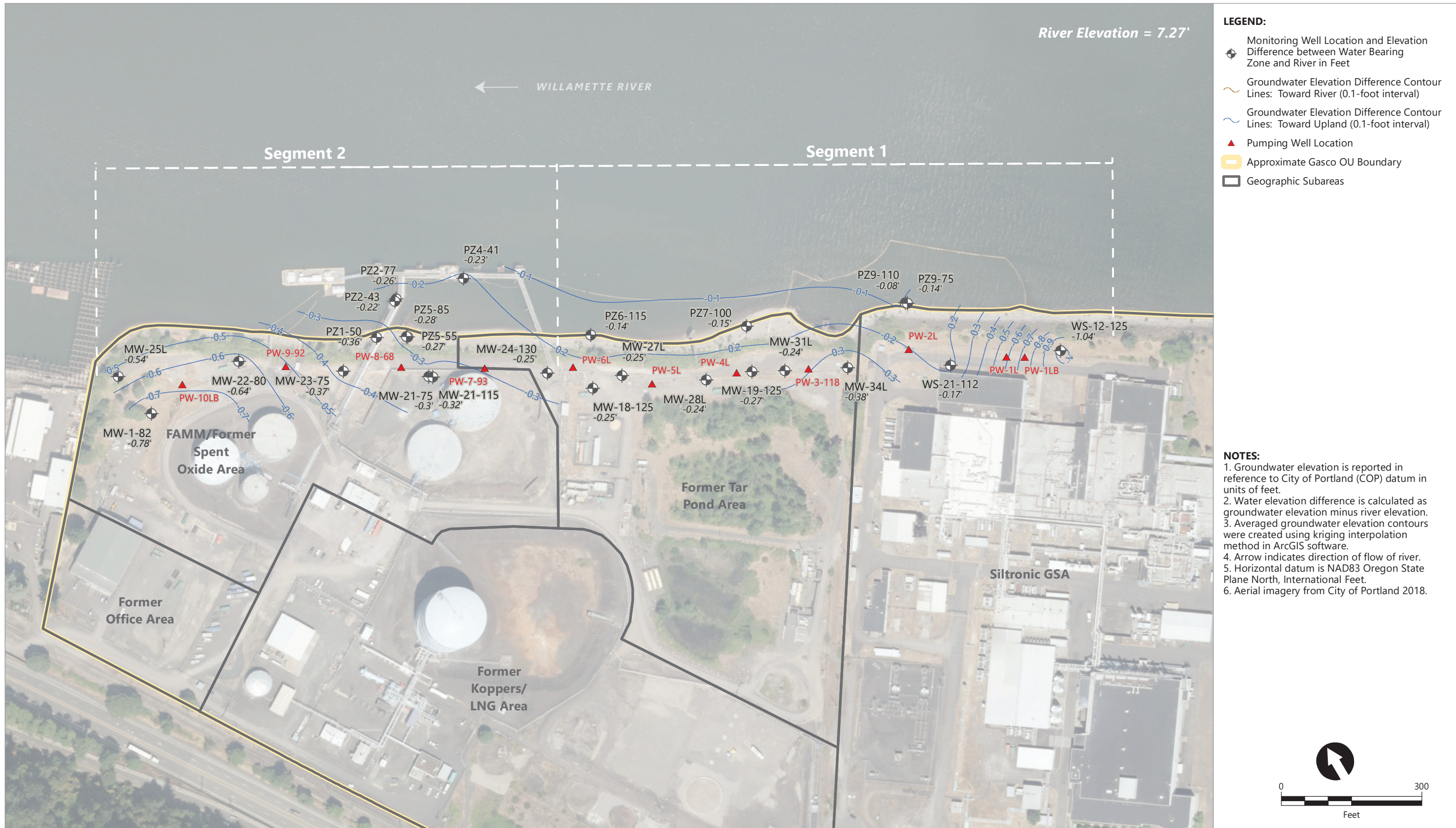
Figure 3.3c Contours of Water Elevation Difference Between Lower Alluvium and River Using Serfes 3-Day Rolling Averages From 3/11/2022-3/13/2022
