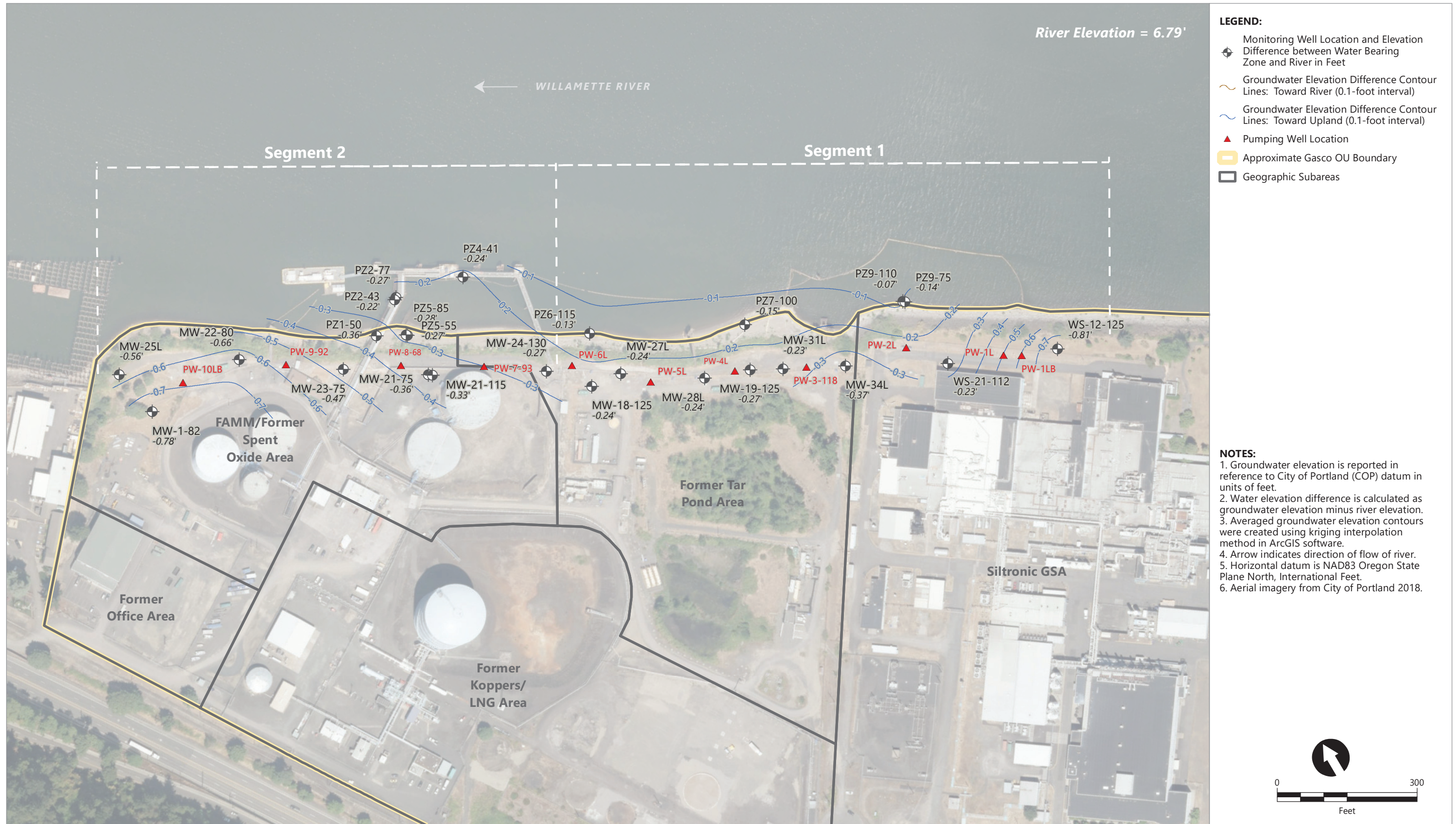
Figure 3.3c Contours of Water Elevation Difference Between Lower Alluvium and River Using Serfes 3-Day Rolling Averages From 4/11/2022-4/13/2022
