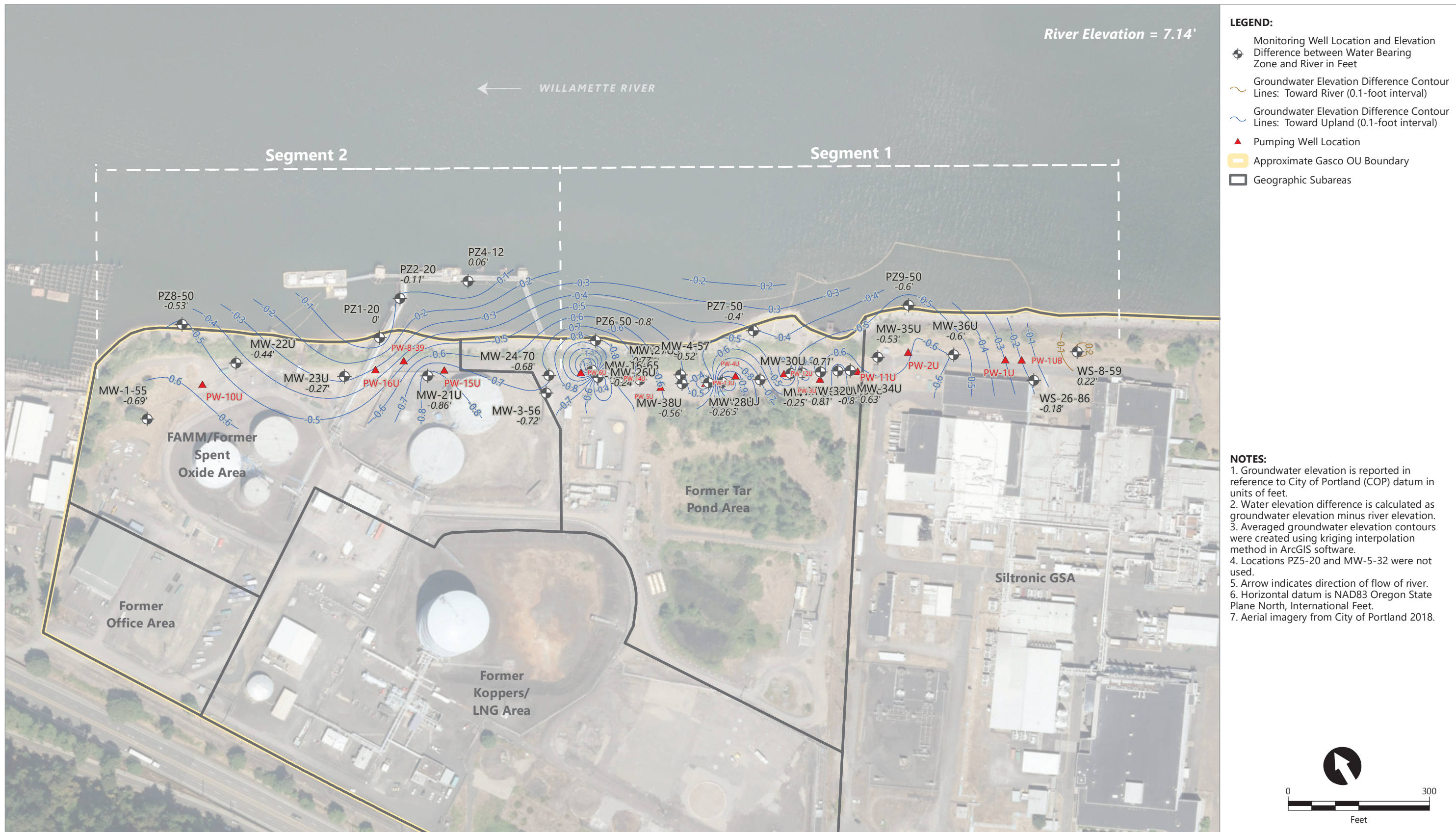
Figure 3.4b Contours of Water Elevation Difference Between Upper Alluvium and River Using Serfes 3-Day Rolling Averages From 3/24/2022-3/26/2022
