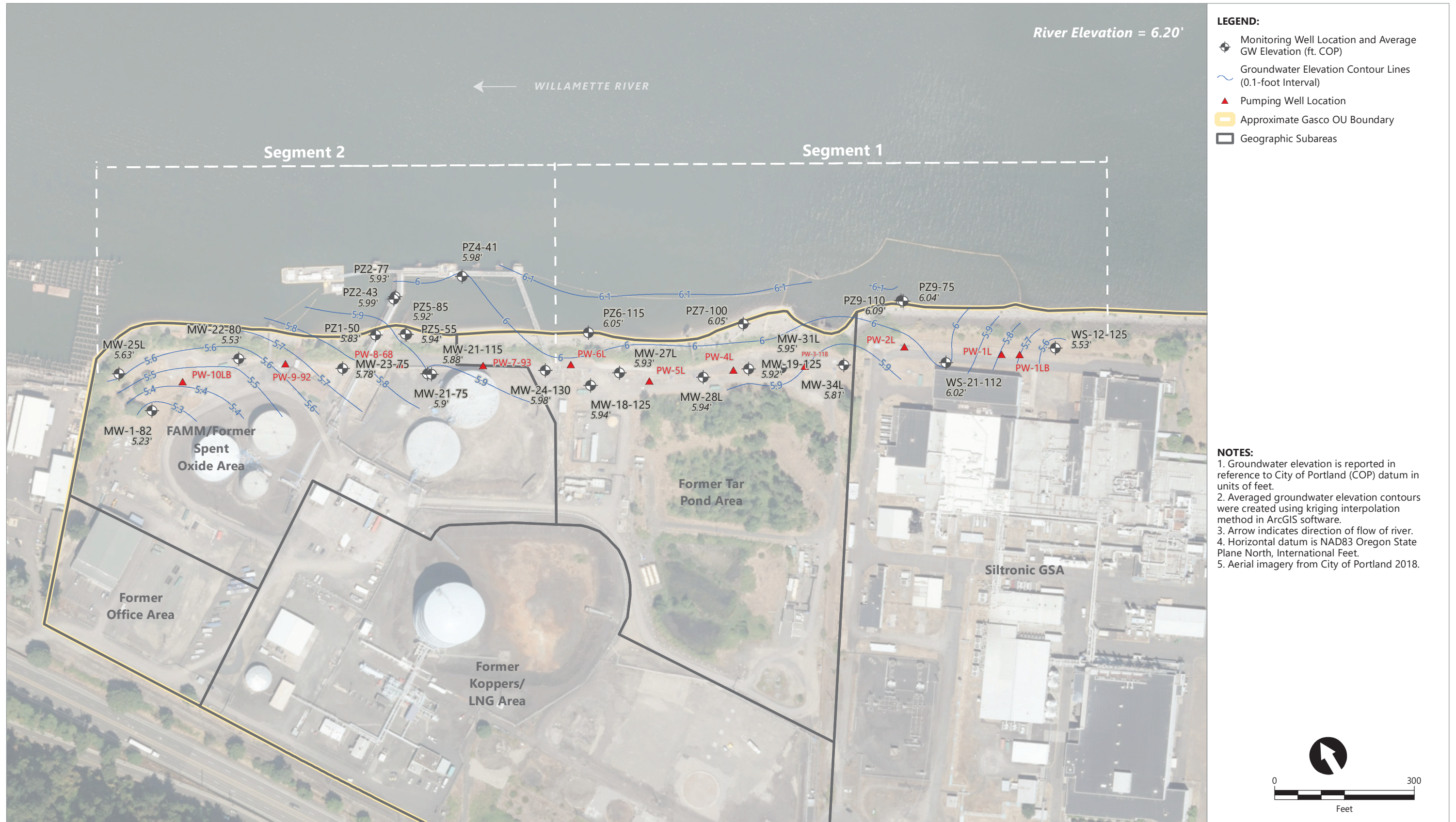
Figure 3.1c Lower Alluvium WBZ Potentiometric Surface Contours Using Serfes 3-Day Rolling Averages From 2/11/2022-2/13/2022
