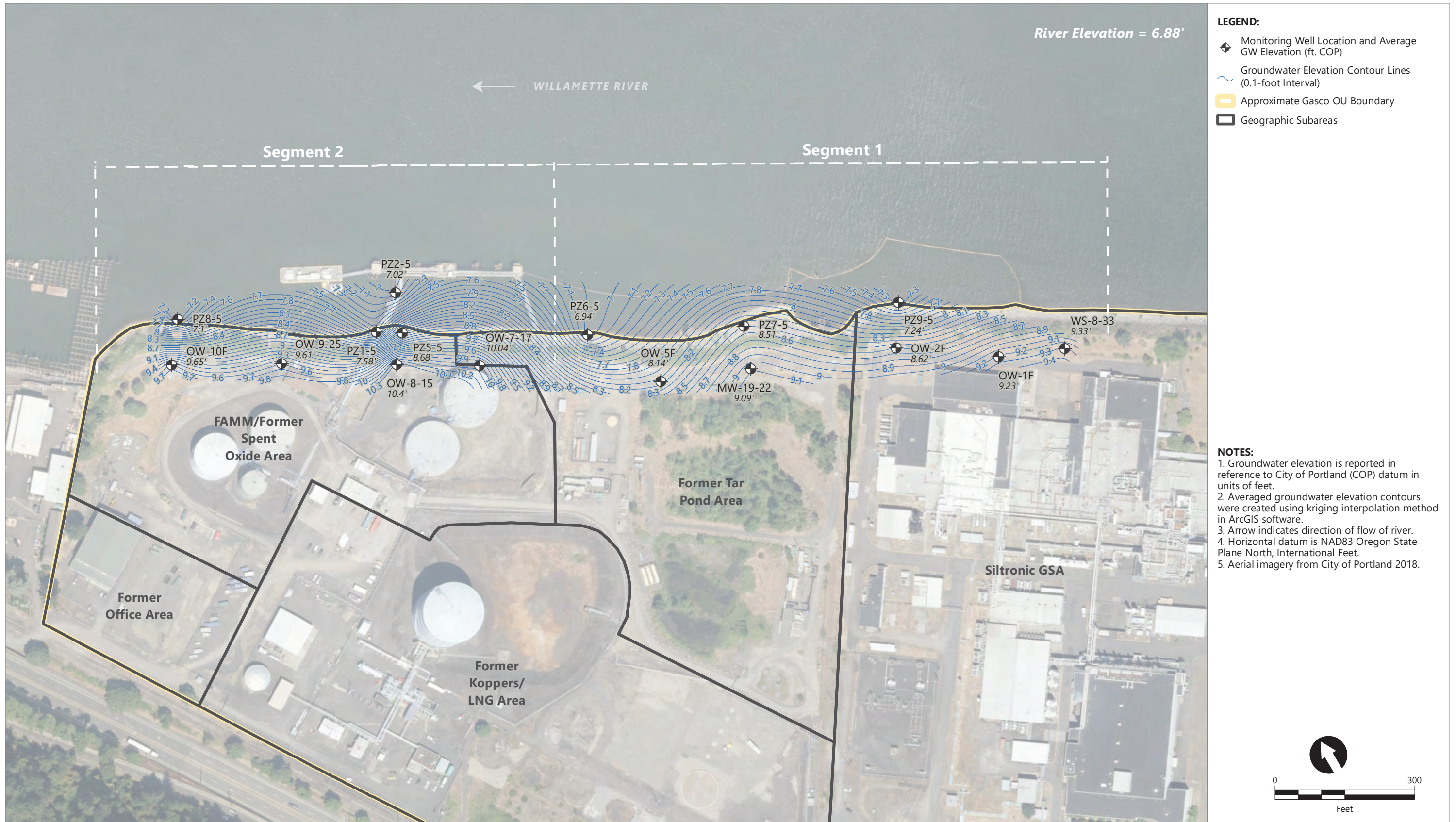
Figure 3.2a Fill WBZ Potentiometric Surface Contours Using Serfes 3-Day Rolling Averages From 7/24/2022-7/26/2022 NWN Gasco Site Portland, Oregon
