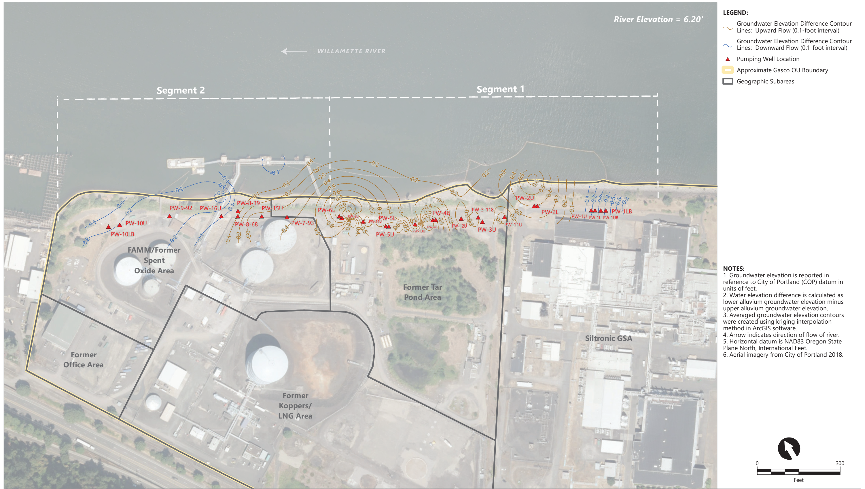
Figure 6.1 Contours of Water Elevation Difference Between Upper and Lower Alluvium Using Serfes 3-Day Rolling Averages From 2/11/2022-2/13/2022
