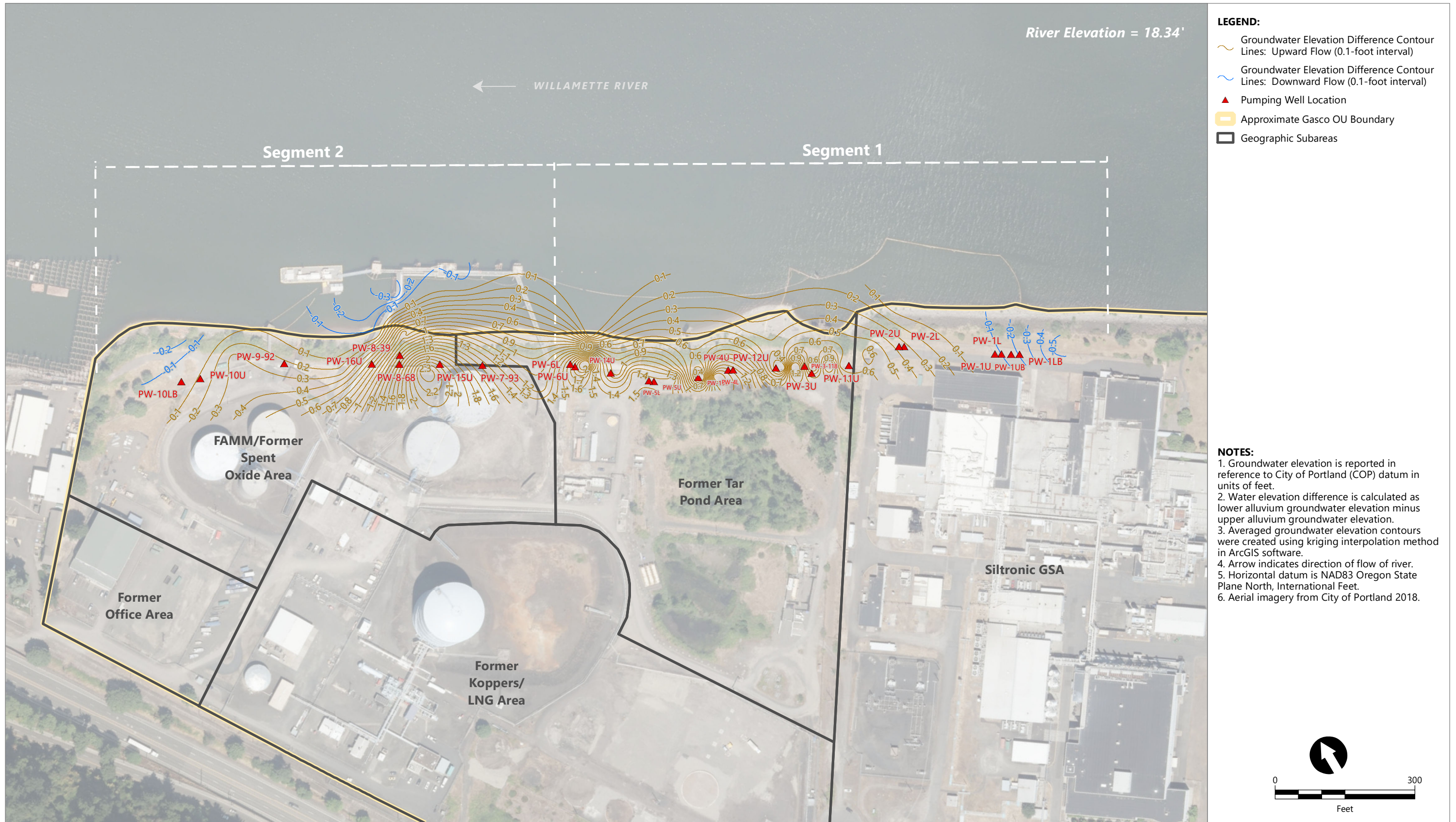
Figure 6.1 Contours of Water Elevation Difference Between Upper and Lower Alluvium Using Serfes 3-Day Rolling Averages From 6/11/2022-6/13/2022
