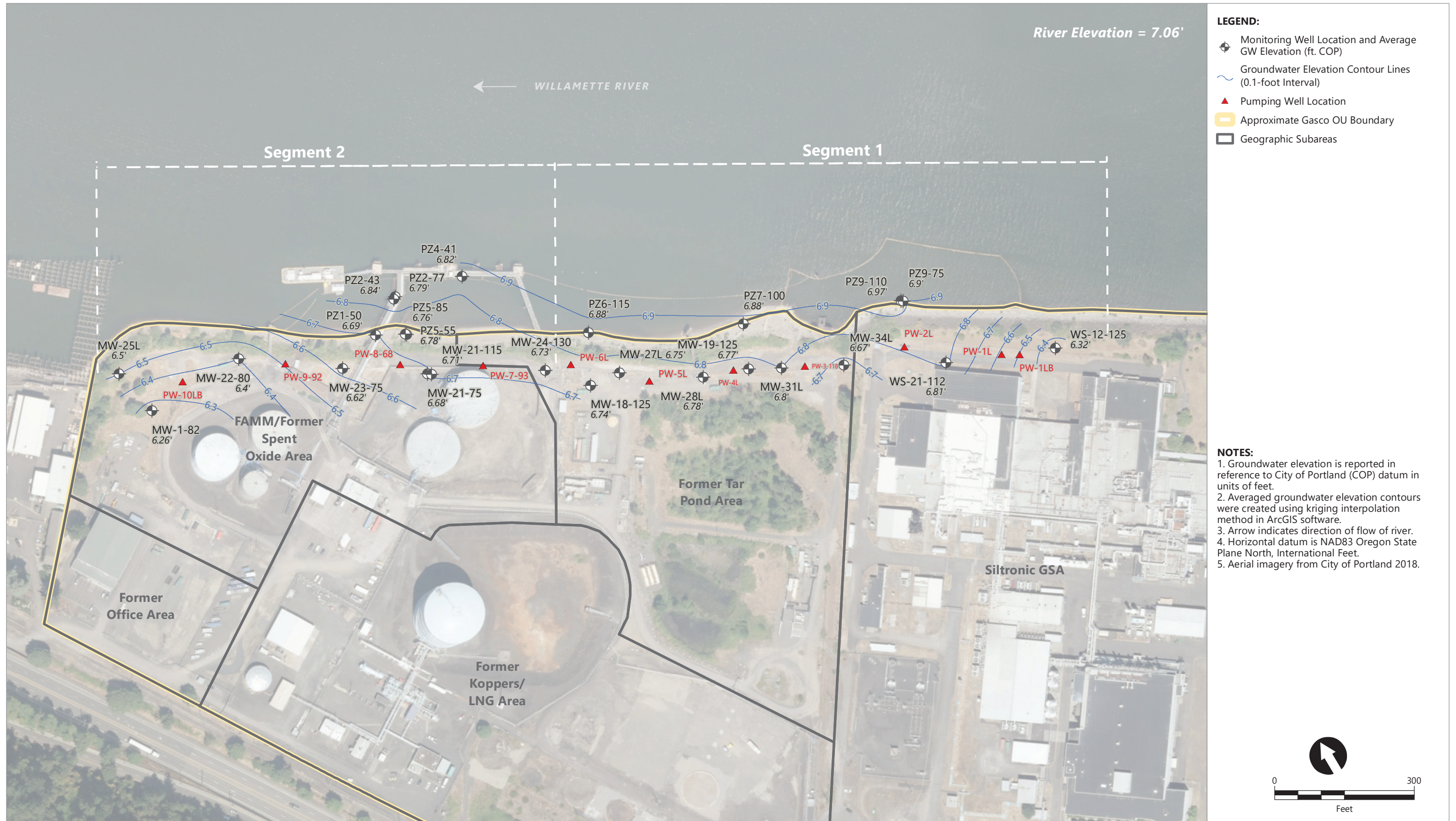
Figure 3.2c Lower Alluvium WBZ Potentiometric Surface Contours Using Serfes 3-Day Rolling Averages From 4/24/2022-4/26/2022
