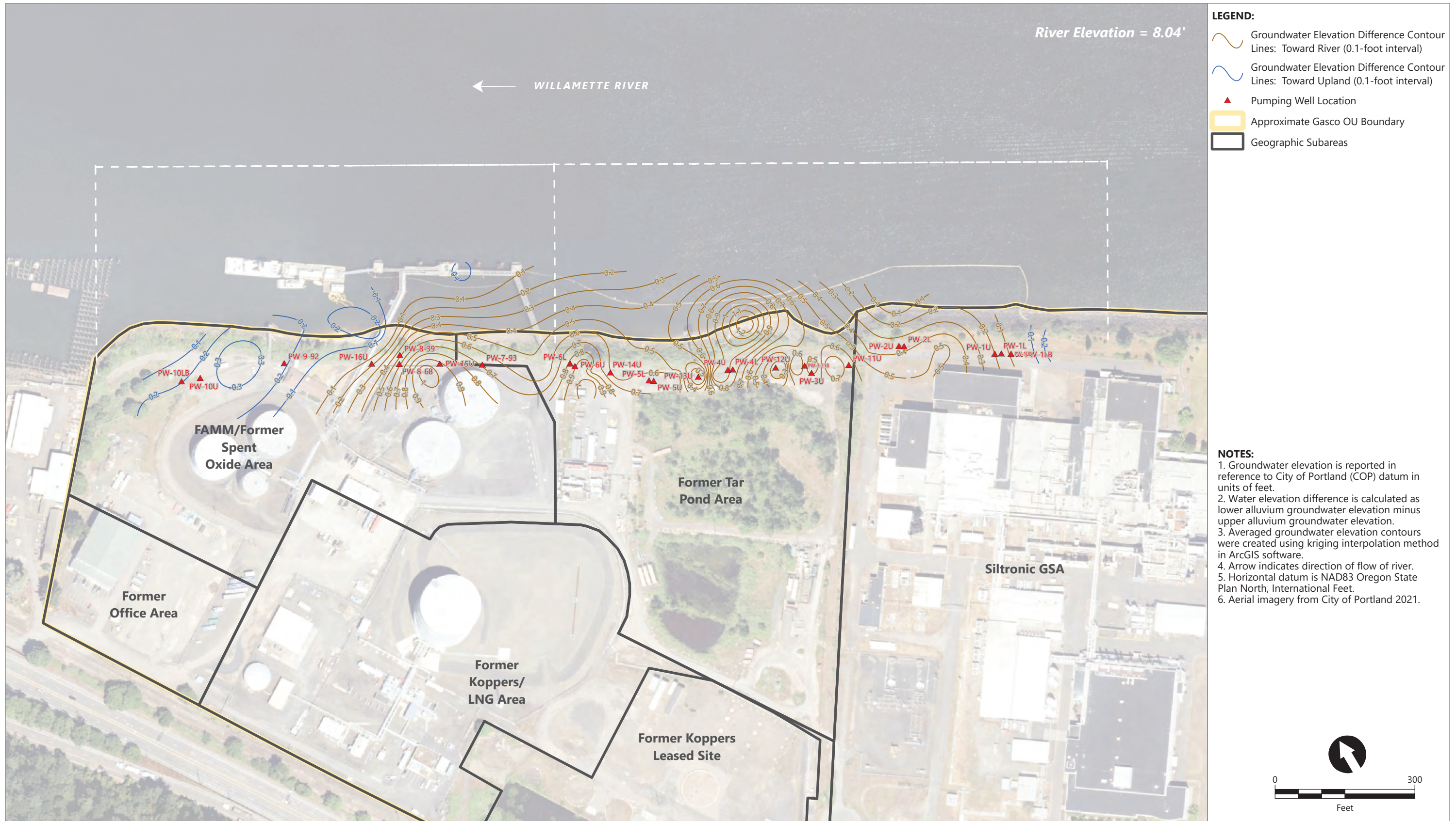
Figure 6.2 Contours of Water Elevation Difference Between Upper and Lower Alluvium Using Serfes 3-Day Rolling Averages From 12/24/2022-12/26/2022
