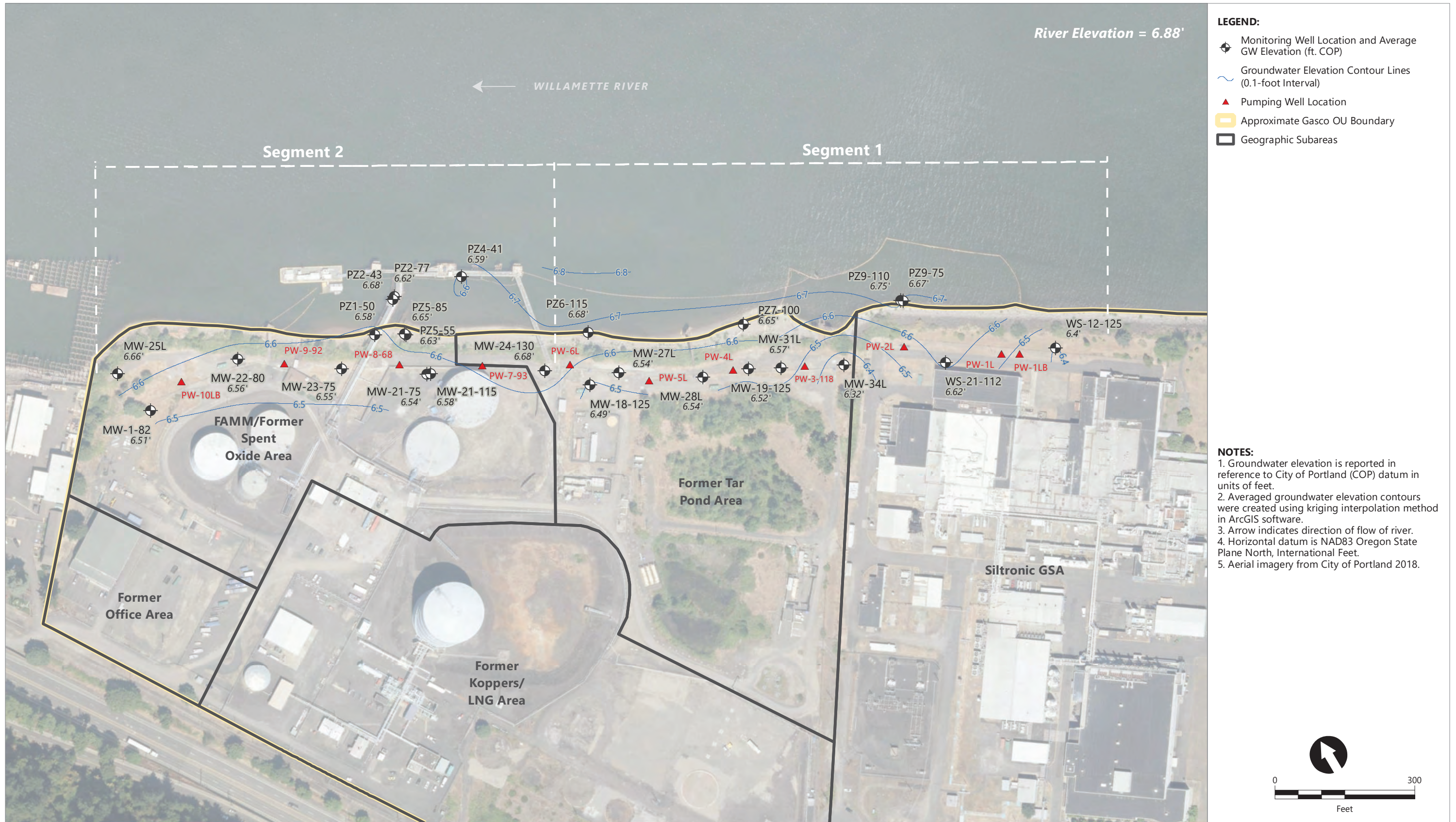
Figure 3.2c Lower Alluvium WBZ Potentiometric Surface Contours Using Serfes 3-Day Rolling Averages From 7/24/2022-7/26/2022
