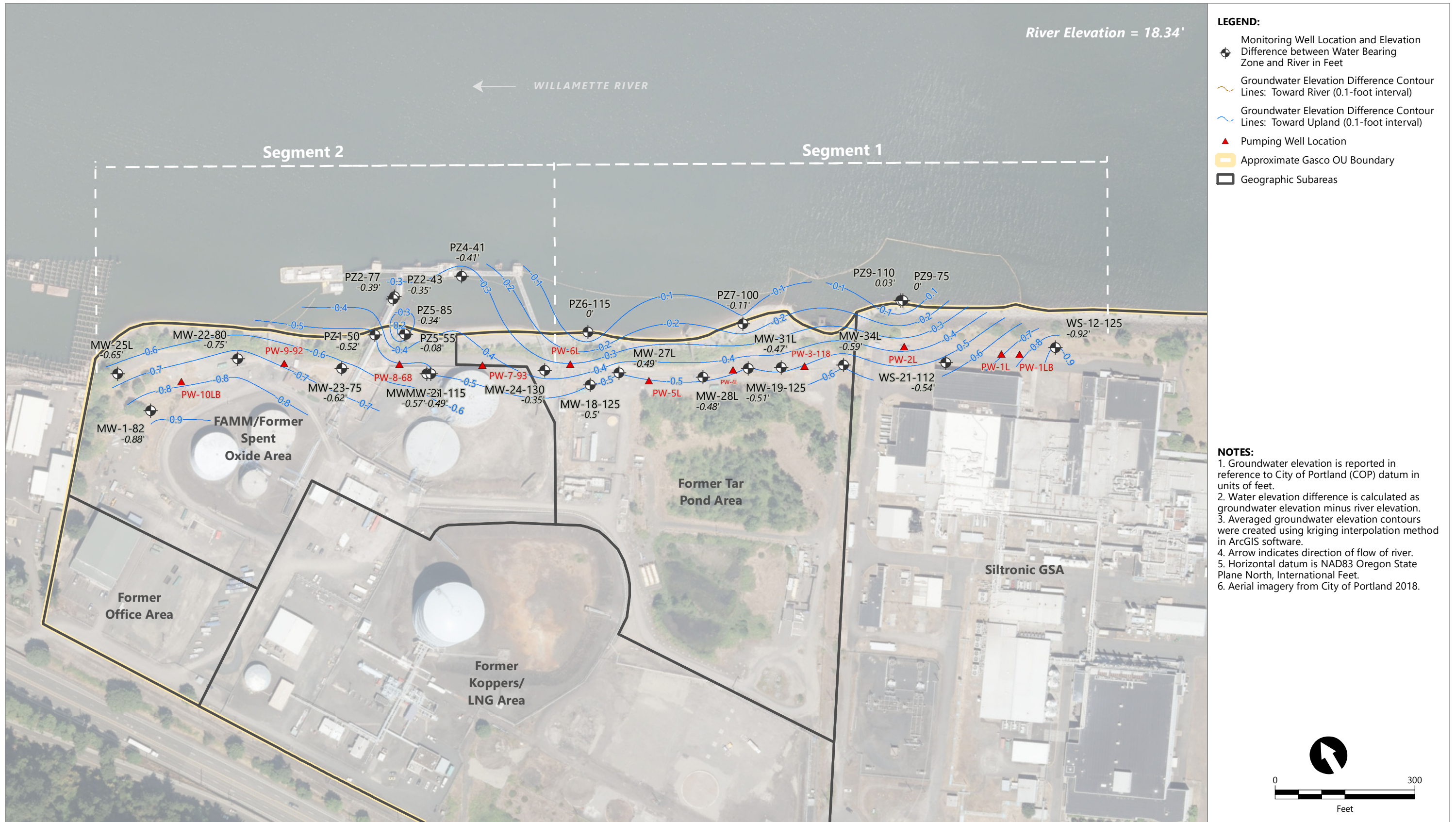
Figure 3.3c Contours of Water Elevation Difference Between Lower Alluvium and River Using Serfes 3-Day Rolling Averages From 6/11/2022-6/13/2022
