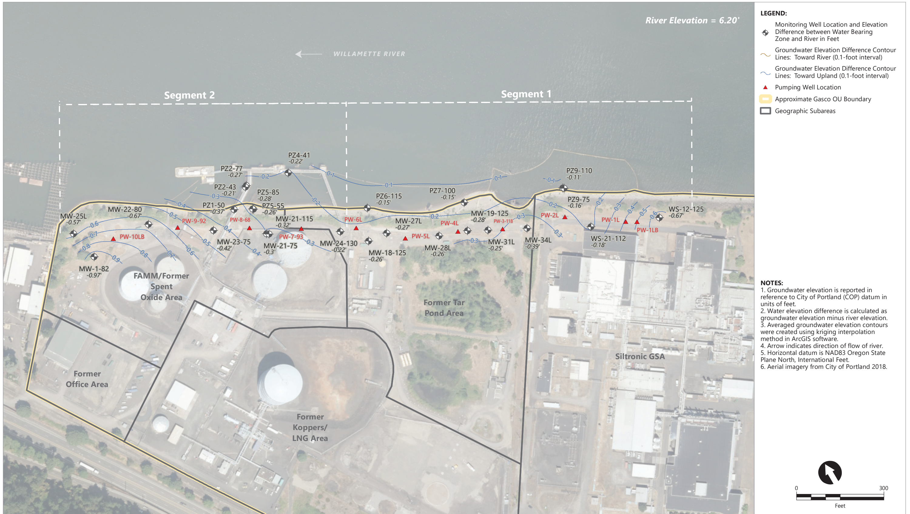
Figure 3.3c Contours of Water Elevation Difference Between Lower Alluvium and River Using Serfes 3-Day Rolling Averages From 2/11/2022-2/13/2022
