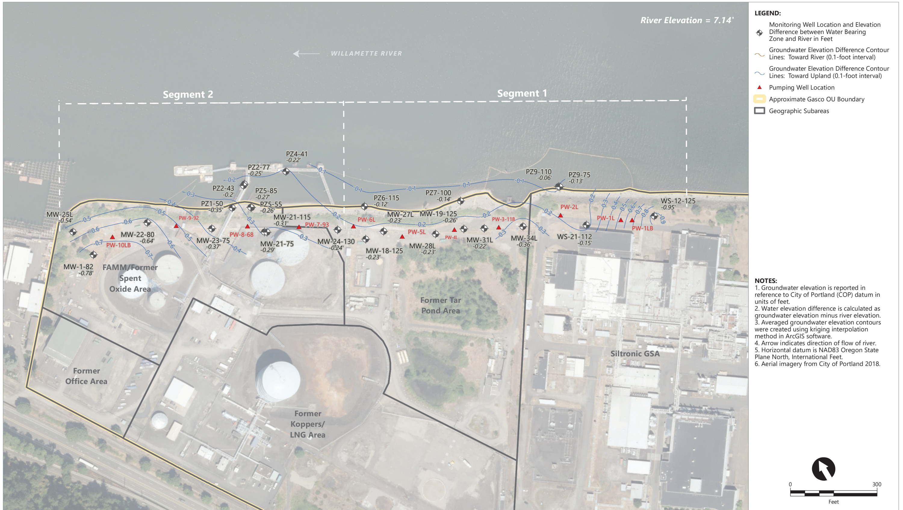
Figure 3.4c Contours of Water Elevation Difference Between Lower Alluvium and River Using Serfes 3-Day Rolling Averages From 3/24/2022-3/26/2022
