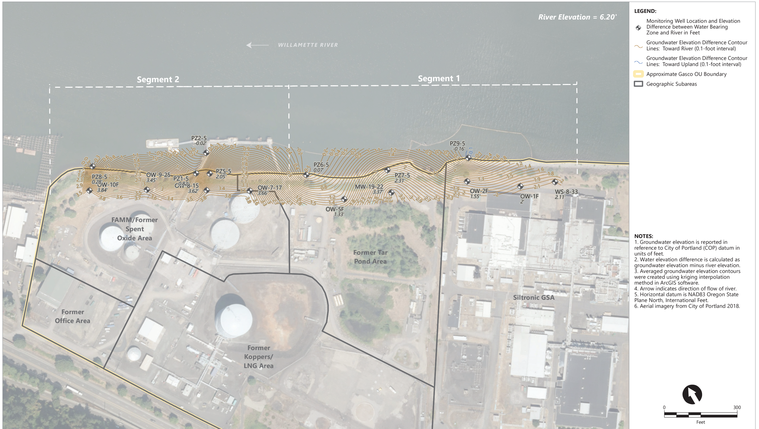
Figure 3.3a Contours of Water Elevation Difference Between Fill and River Using Serfes 3-Day Rolling Averages From 2/11/2022-2/13/2022
