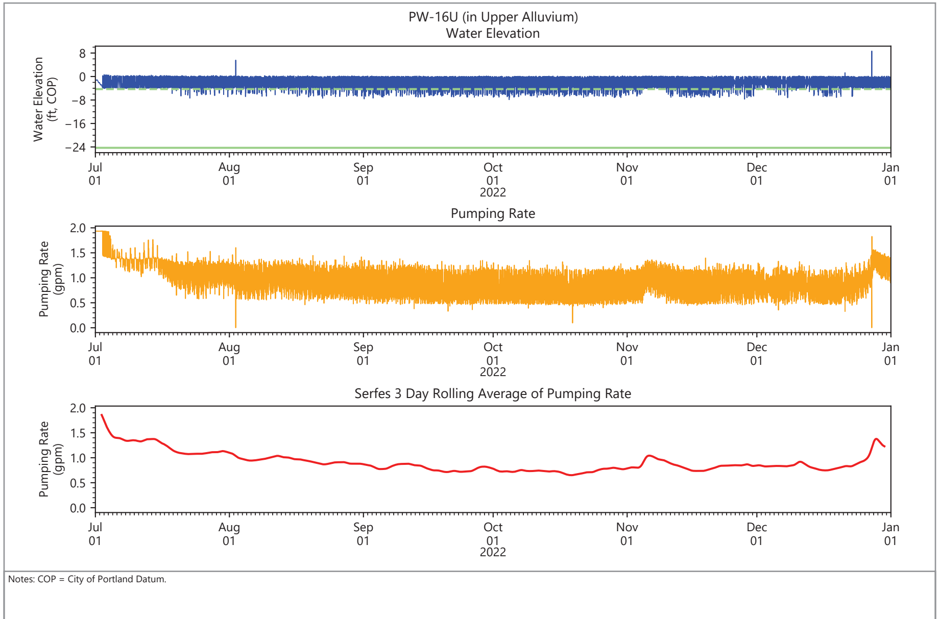
Figure 8.16 Groundwater Elevations and Pumping Rates at Pumping Wells NW Natural Gasco Site
