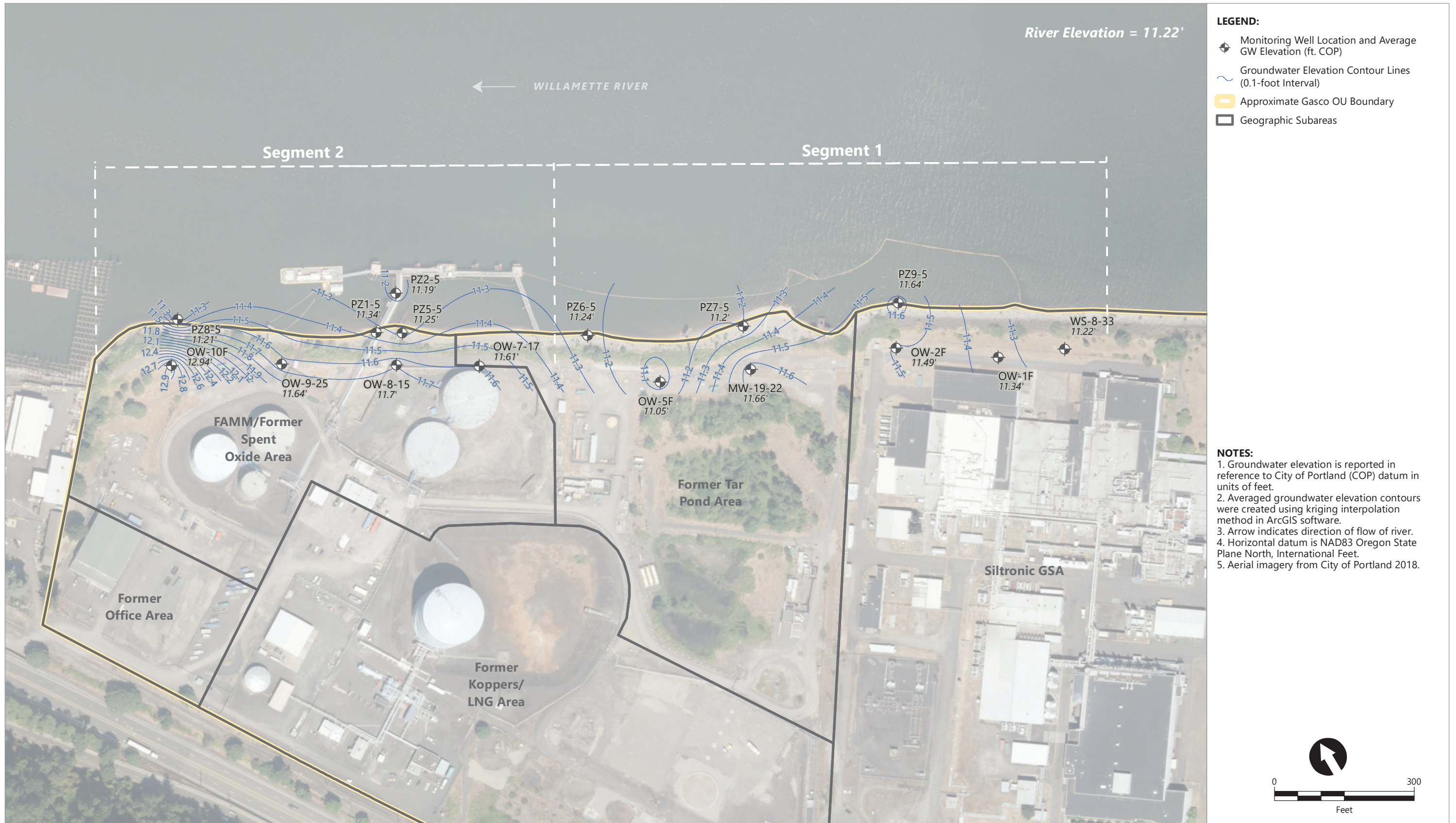
Figure 3.1a Fill WBZ Potentiometric Surface Contours Using Serfes 3-Day Rolling Averages From 5/11/2022-5/13/2022
