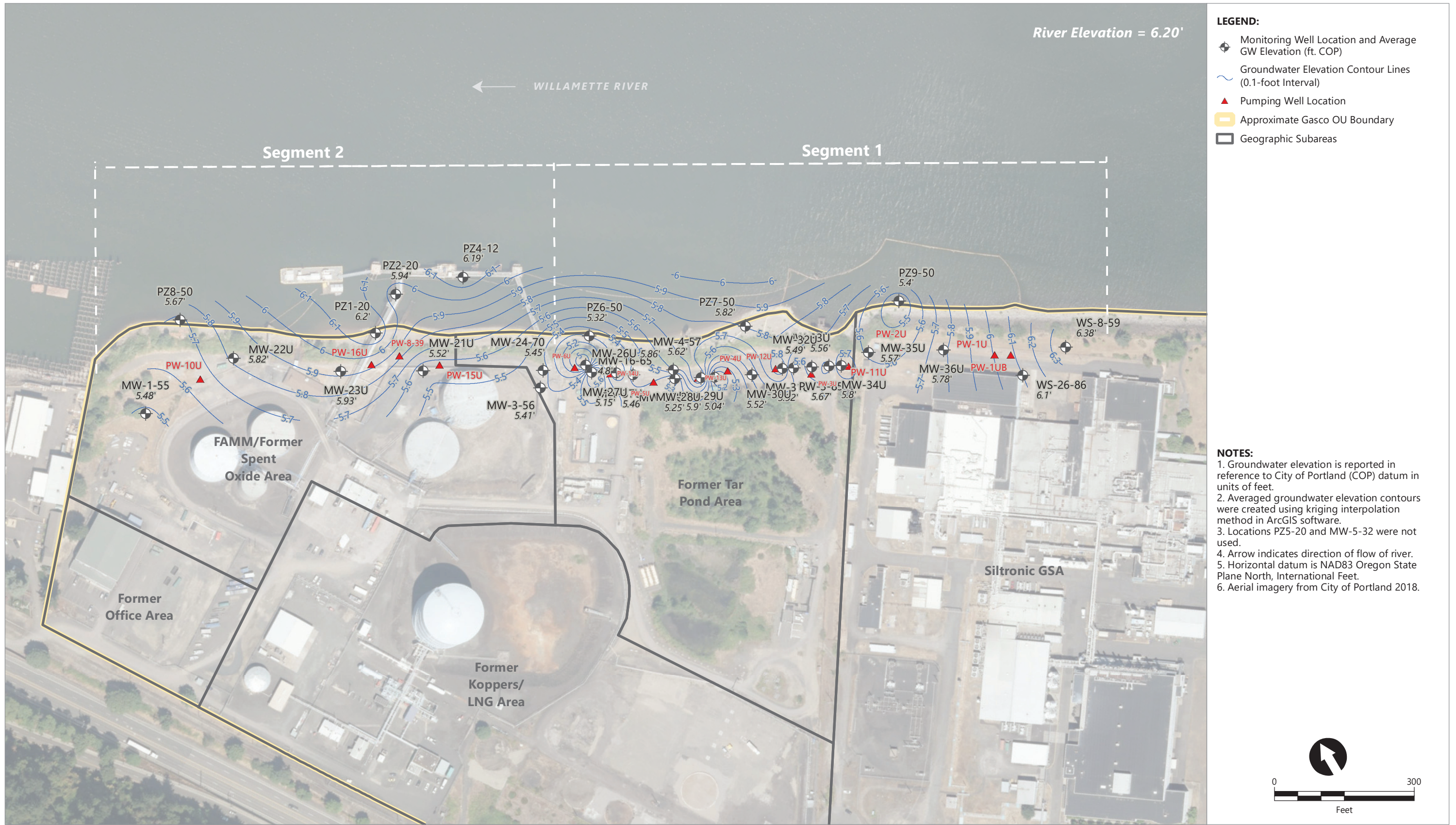
Figure 3.1b Upper Alluvium WBZ Potentiometric Surface Contours Using Serfes 3-Day Rolling Averages From 2/11/2022-2/13/2022
