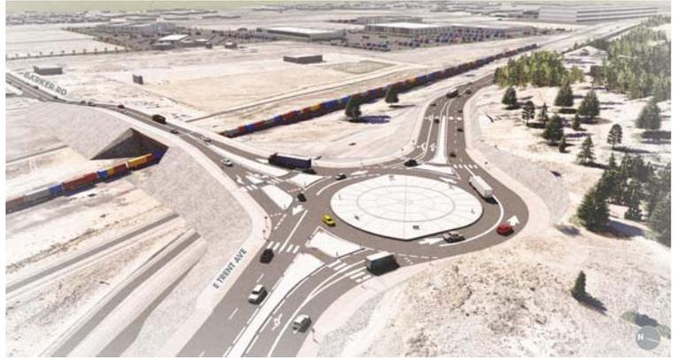
At the adjacent intersection of Barker Road and Trent Avenue, a two-lane roundabout will be constructed to improve safety at the intersection. The Washington State Department of Transportation will provide construction oversight of both the grade separation and intersection work.
