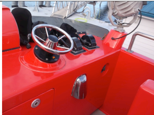
10 Flying Bridge Control Console
