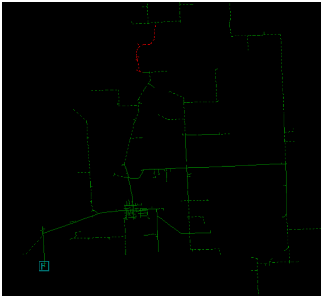
WIL12F2 – Several sections showing low voltage. This will be fixed by the grid modernization work.
