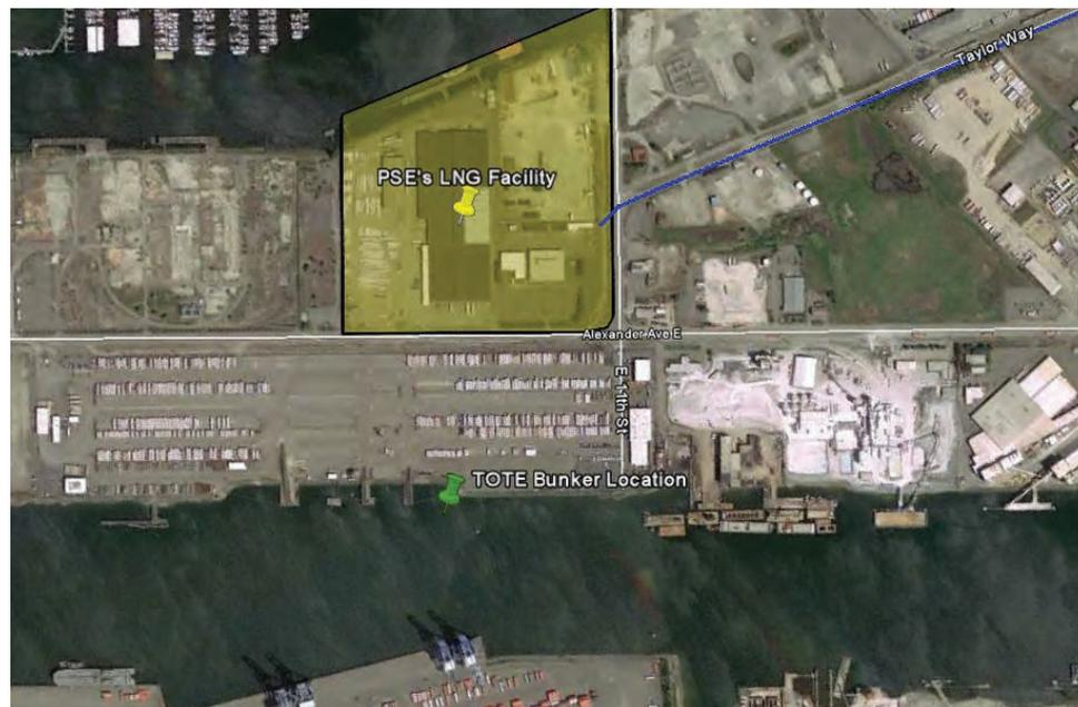
This location meets all the inherent requirements previously discussed, and allows PSE to meet the peak-day needs of gas customers by connecting to PSE's high pressure distribution system with approximately four miles of 16-inch pipe that will be constructed predominately inside the Port of Tacoma.
