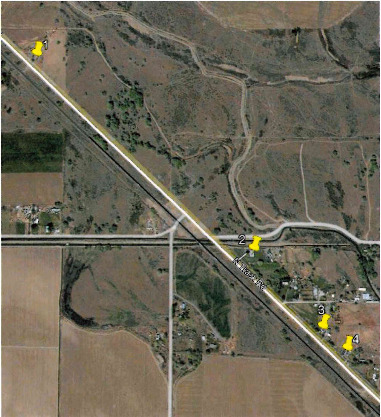
Figure 2: Section of the proposed pipeline showing buildings 1-4 within the 100-foot proximity boundary.
