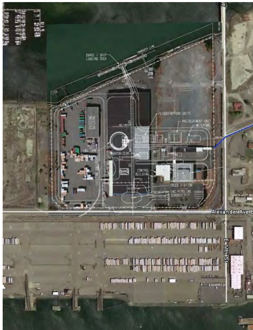
Figure 1. Tacoma LNG Facility Plot Plan
