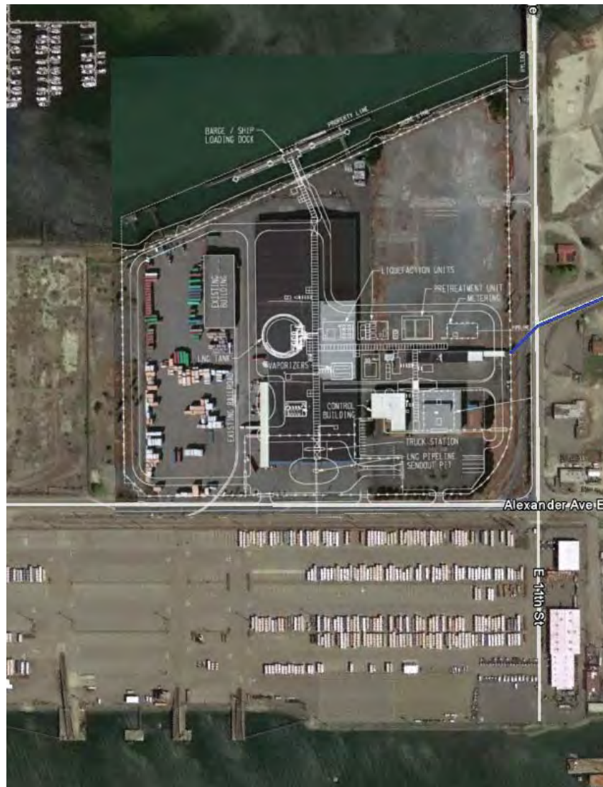
Figure 1. Tacoma LNG Facility Plot Plan
