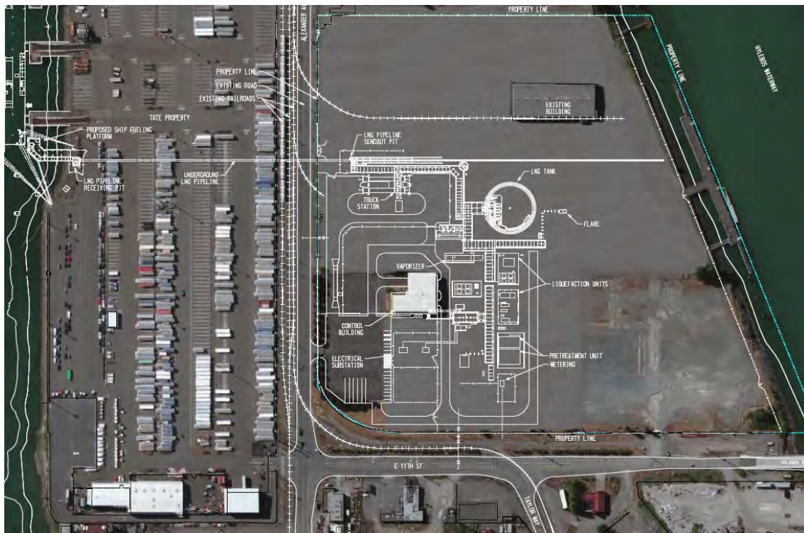
Figure 1. Tacoma LNG Facility Plot Plan
