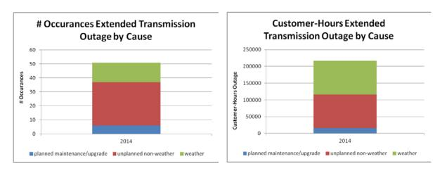
Figure 5: Transmission outage causes affecting customers in 2014
