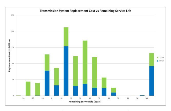
Figure 3: Replacement Cost vs. Remaining Service Life
