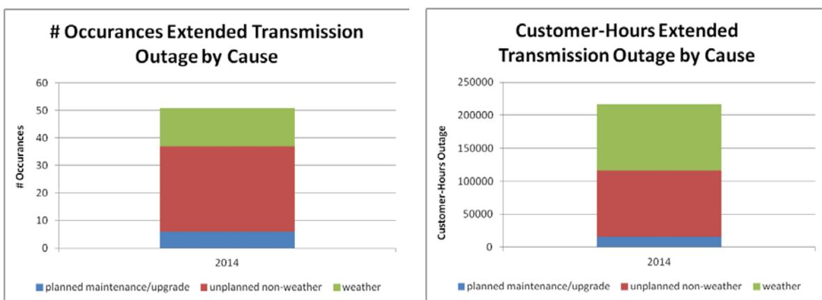
Figure 5: Transmission outage causes affecting customers in 2014
