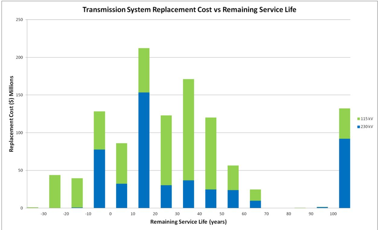
**Figure 3: Replacement Cost vs. Remaining Service Life**
