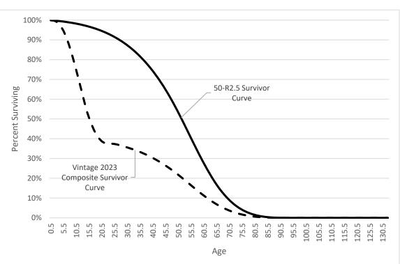
The solid black line shows the 50-R2.5 survivor curve estimate. The dashed line shows the result of combining this estimate with retirements from downsizing the gas system. Once these retirement ratios are combined and a composite Life Cycle curve is developed, average service lives and remaining lives can be calculated using the same methods as for an Iowa survivor curve.<sup>9</sup>
