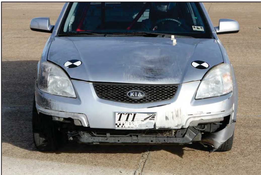
Figure 1.3. Kia Rio (MASH Test Vehicle) after 100 Impacts.
