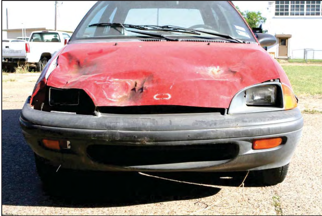
Figure 1.2. Geo Metro (NCHRP Report 350 Test Vehicle) after Approximately 50 Impacts.
