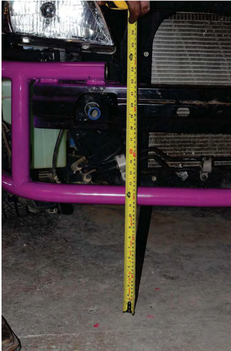
Figure 4.4. Modified Bumper Ground Clearance.
