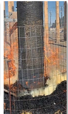
A controlled burn test using the mesh wrap
