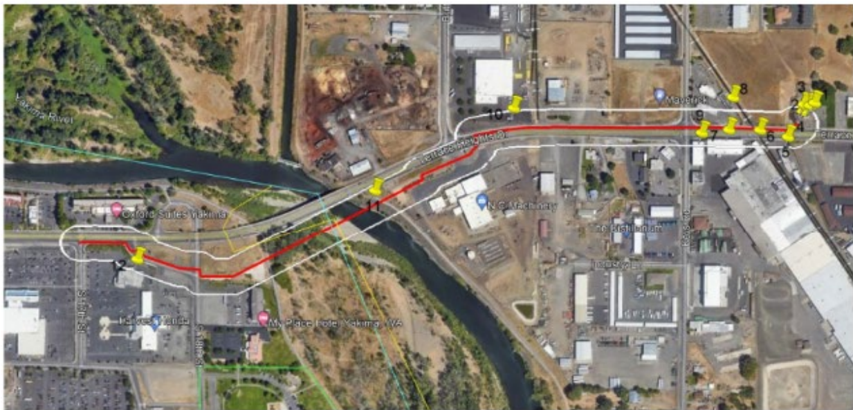
Figure 2: Section of the proposed pipeline showing buildings 1-12 within the 100-foot proximity boundary.
