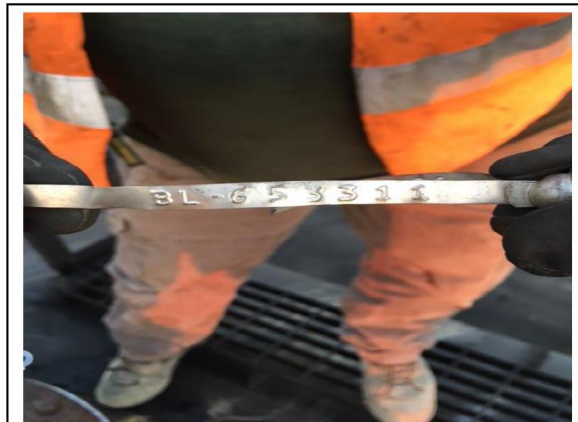
Photo 4: Custody seal removed from manway.
