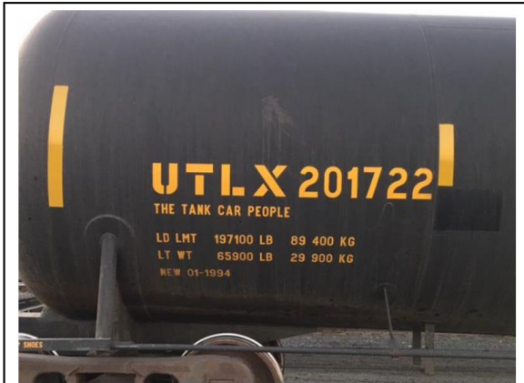
Photo 1: Tank car identification markings.
