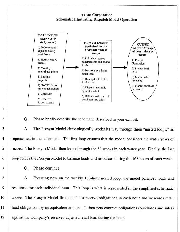
Second, the Prosym Model dispatches hydroelectric projects to flatten the overall load shape while still meeting minimum flow requirements. This step utilizes the flexibility of the hydroelectric system to meet peak load requirements.
