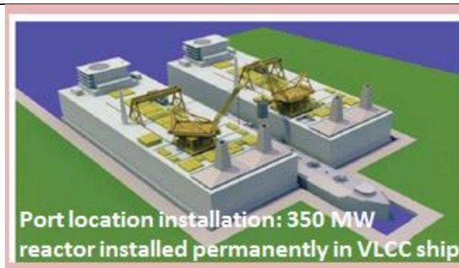
Illustration 11. Design of a 350 MW Gen IV molten salt reactor (Thorcon, Seattle)
