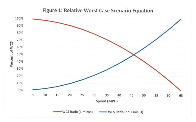
Figure 1 demonstrates the relationship of speed to the percentage of train applicable to proposed insurance coverages. Kinetic energy =  $\frac{1}{2}$  Mass x (Velocity)<sup>2</sup> and PHSMA assumes loaded HHFT's are of equal mass.
