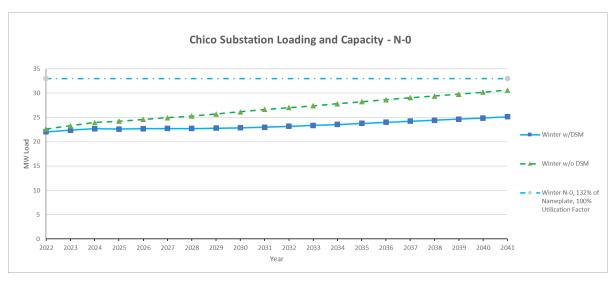
Figure 3-3: Chico Substation N-0 Capacity
