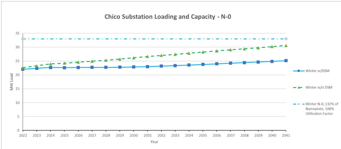
Figure 3-3: Chico Substation N-0 Capacity
