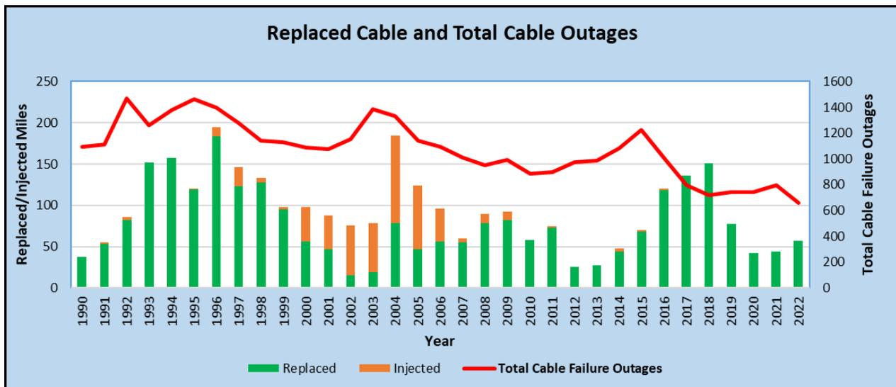
The majority of cables have been remediated through replacement; however, a smaller population were injected with silicone to remediate the insulation issue and extend the life of the cable. Since 2016, the plan has focused on replacement, which has delivered notable reduction in cable failures.
