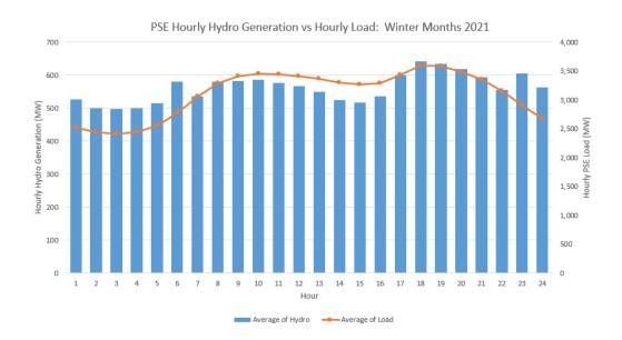
The following figure demonstrates how PSE shaped its hydro generation to meet its hourly load during Winter 2021.
