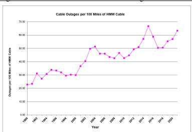
Figure 1: HWM Cable Failure Caused Outage Per 100 Miles
