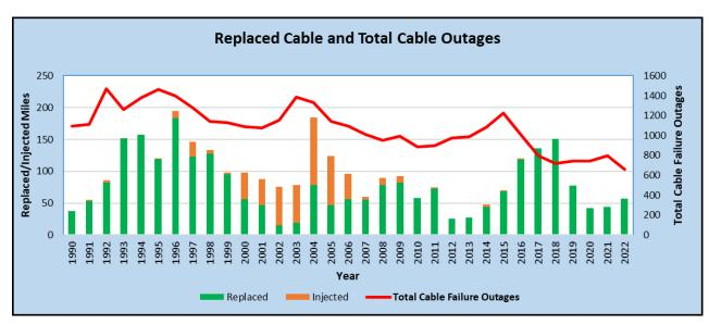
Figure 2: 1990 – 2022 Annual Cable Failure Outages and Miles of Remediated Cable
