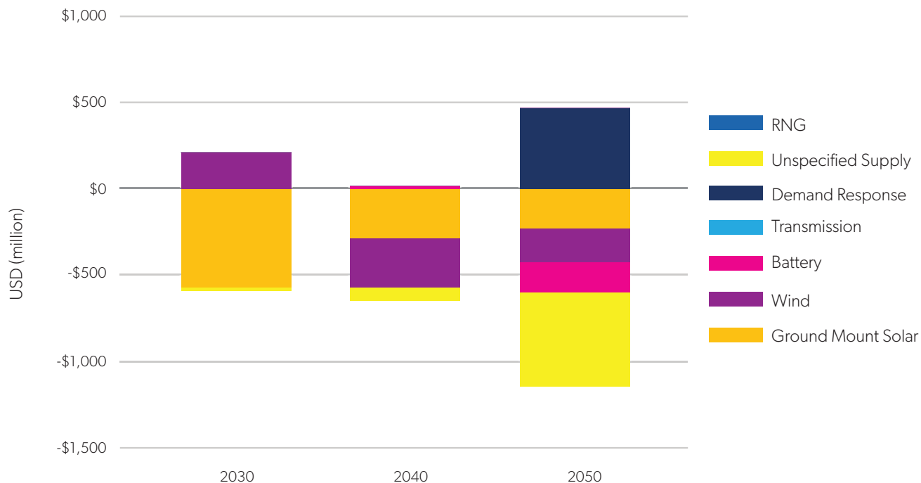
Figure 93. Incremental capital costs for developing energy supply in the Electrification scenario, relative to the BAP.
