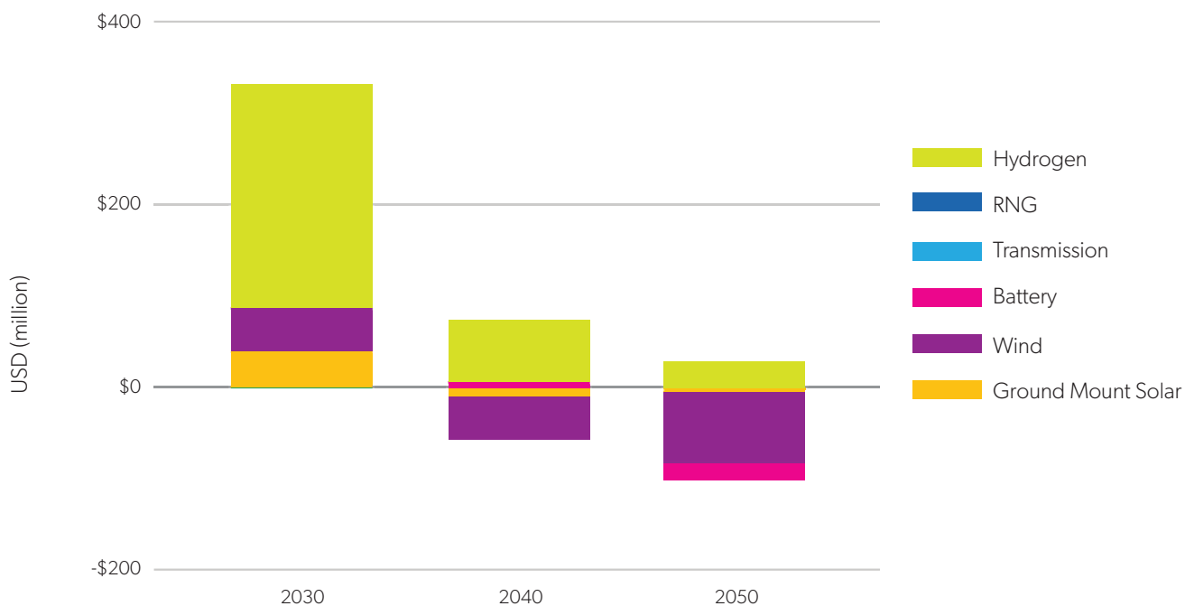
Figure 97. Incremental operating and maintenance costs in 2030, 2040, and 2050 to meet electricity demand in the Alternative Fuels scenario, relative to the BAP.
