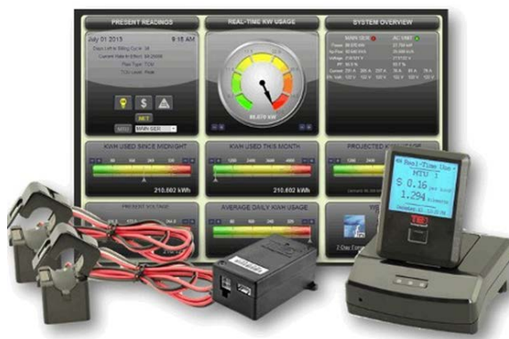
Figure 2-16. Example Energy Monitoring System (Clauser, 2016)
