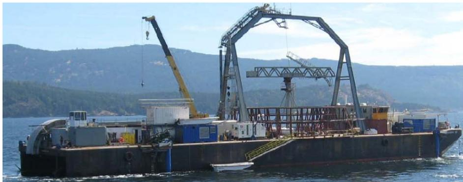
**Figure 16: Typical lay-barge with dynamic positioning for 230 kV cable laying**
