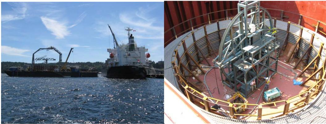
*Figures 10 and 11: Cable transfer from freighter to lay-barge; cable in hold of freighter prior to transfer*
