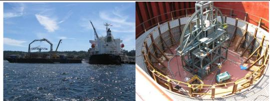
Figures 10 and 11: Cable transfer from freighter to lay-barge; cable in hold of freighter prior to transfer
