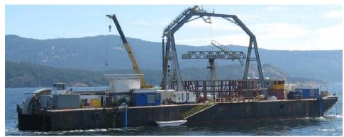
Figure 16: Typical lay-barge with dynamic positioning for 230 kV cable laying
