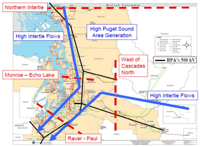
Figure 6-2: Summer Power Flow Resulting from Northern Intertie
