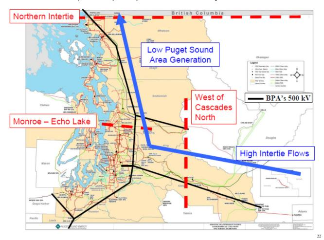
Figure 6-1: Winter Power Flow resulting from Northern Intertie
