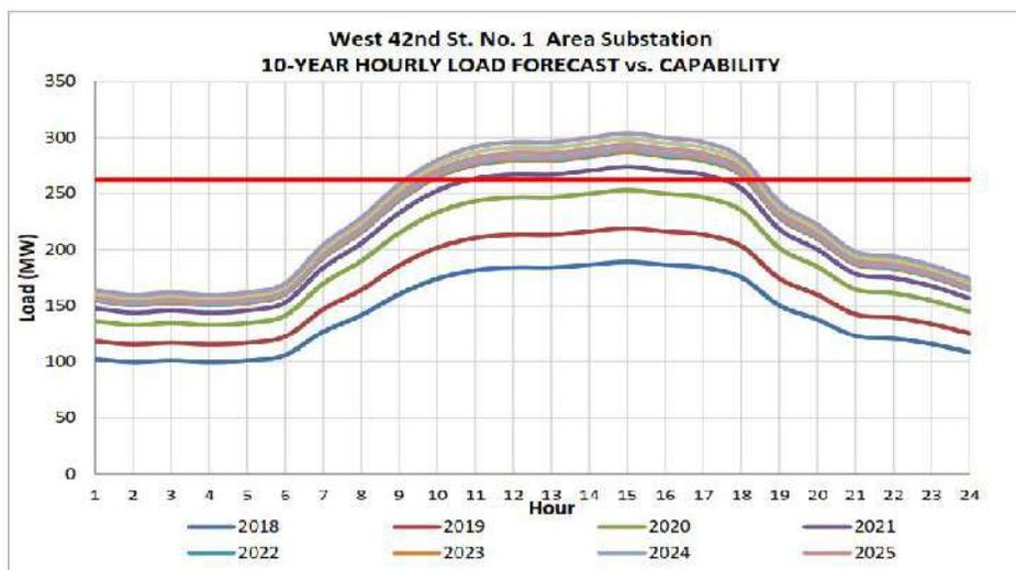
Figure 36: ConEd's 42nd Street Transfer Project Overload Profiles
