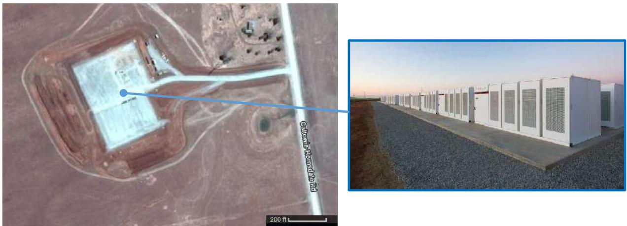
Figure 31: Hornsdale Power Reserve (100MW/129MWh) is approximately 2 hectares in size<sup>83</sup>
