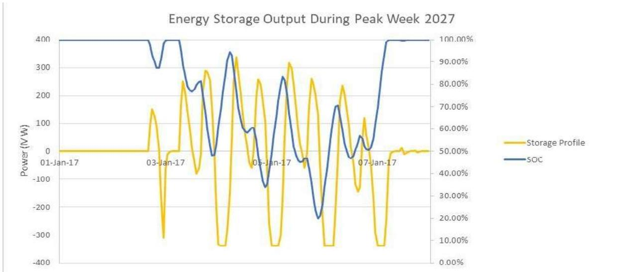
Figure 6: Output of the Complete Solution during the peak week, 338MW/3,679MWh (10.9-hour system)
