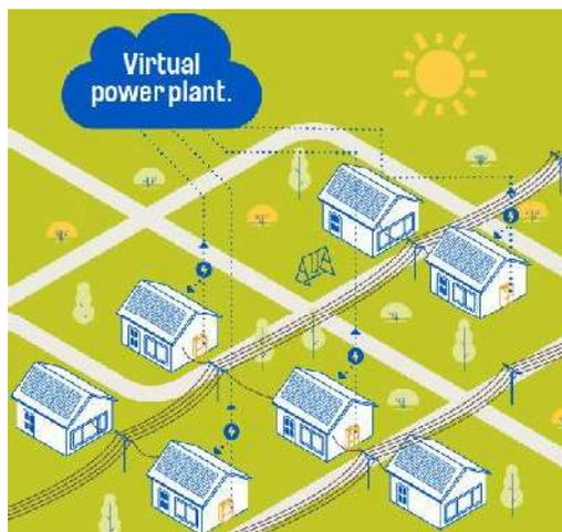
Figure 33: Diagram of the VPP utilizing dispersed PV coupled energy storage to provide aggregated grid benefits<sup>96</sup>
