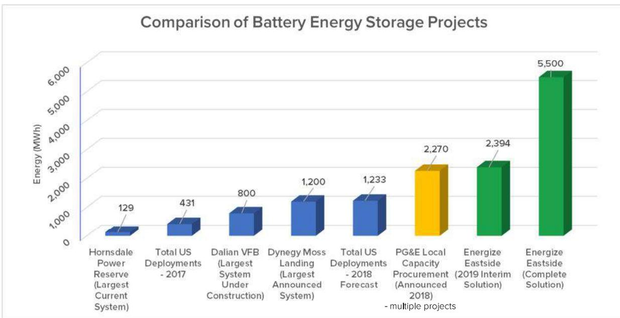
Figure 1: An energy storage system to solve the Eastside constraint in comparison to other projects<sup>20</sup>
