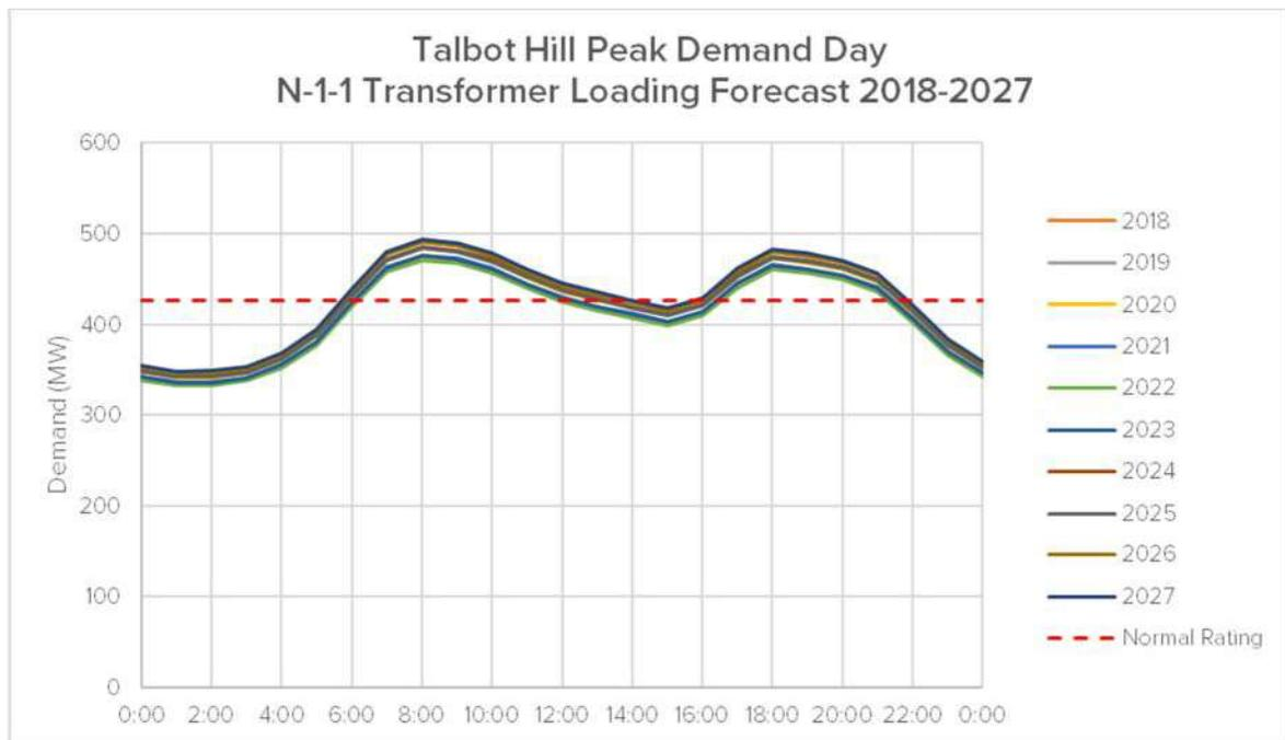
Figure 21: Peak demand loading forecast from 2018 to 2027
