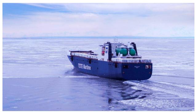
North Star was fitted with two 1,100 m3 LNG tanks for its conversion
