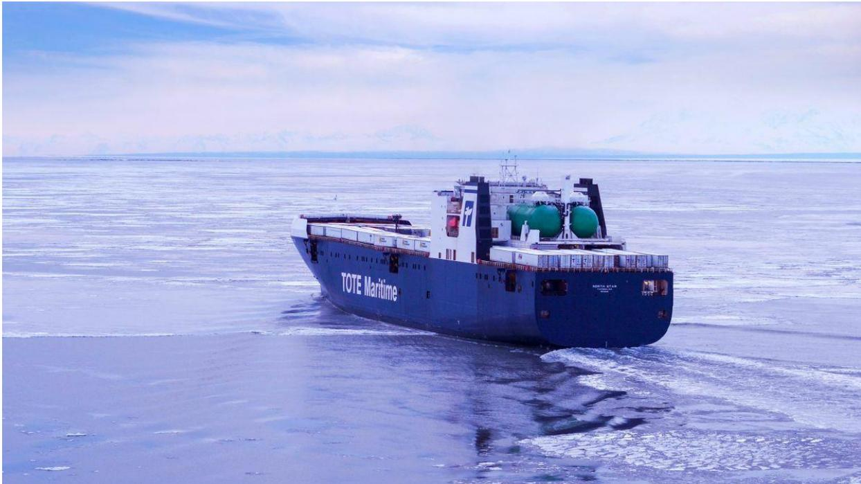
North Star was fitted with two 1,100 m3 LNG tanks for its conversion
