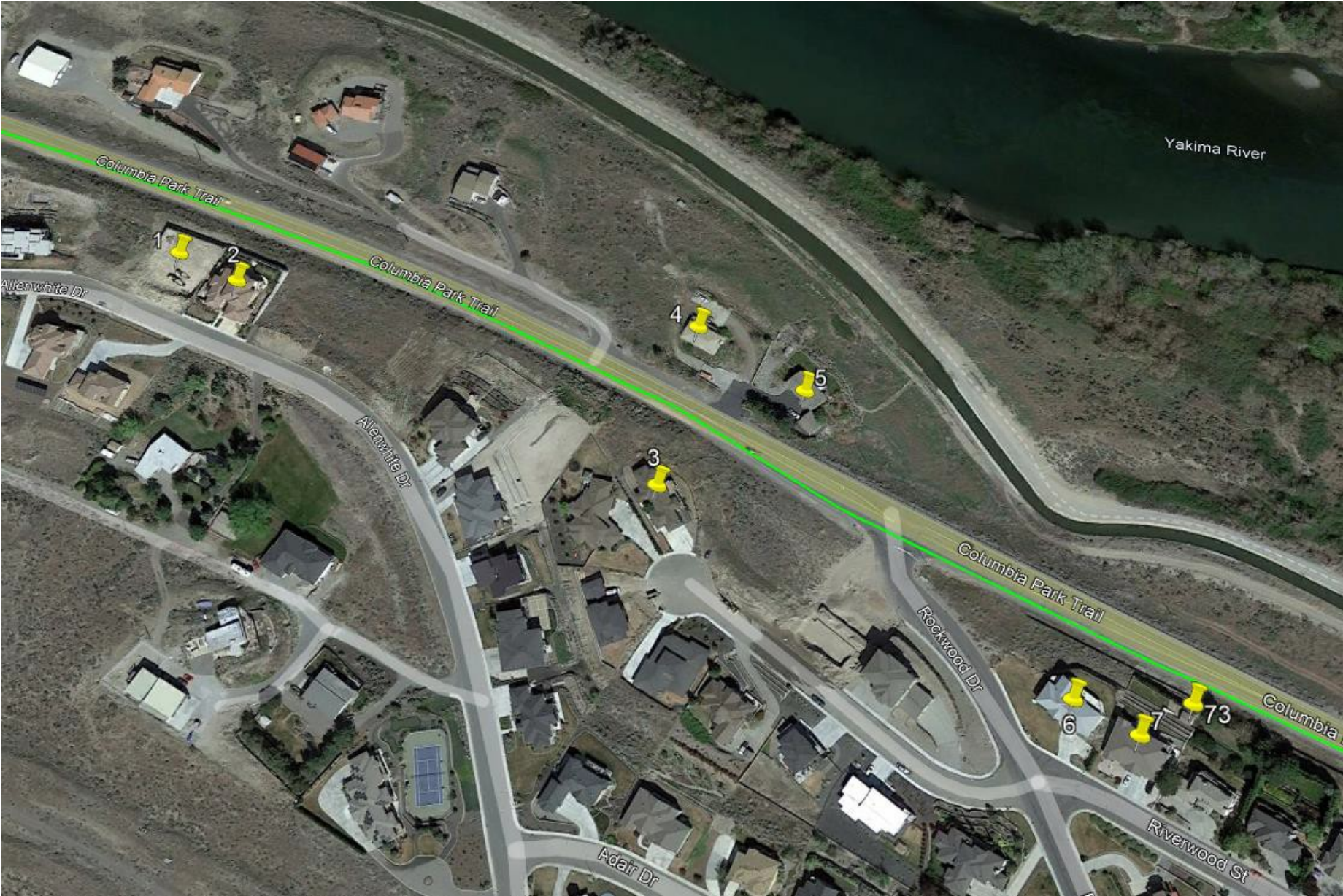
Figure 2: Section of the proposed Richland HP Lateral showing its proximity to buildings 1-7 & 73 within the 100-foot boundary.
