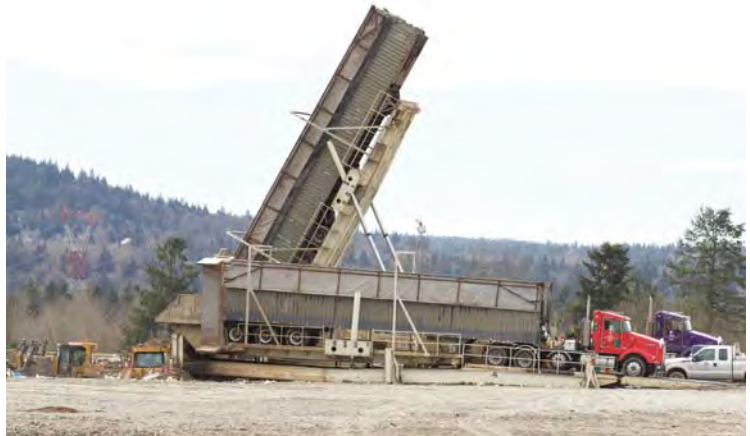
Landfill tippers are an efficient way to empty transfer trailers.
