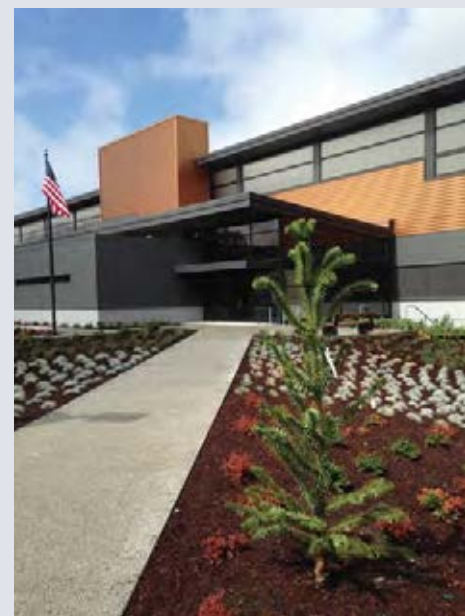
Factoria drought-tolerant plants and permeable pavement
