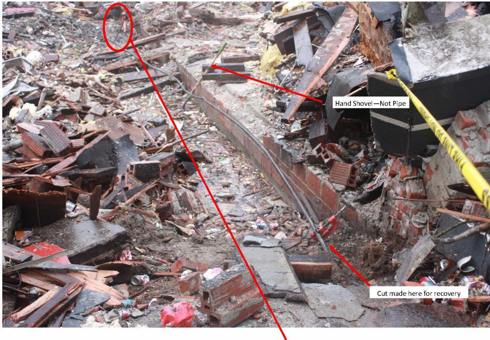
Image 24. Circled region of photo shows riser that fed 8409 and 8411 Greenwood Avenue North, with the dual “twin” service branching off to what is now 8415 Greenwood Avenue North.
