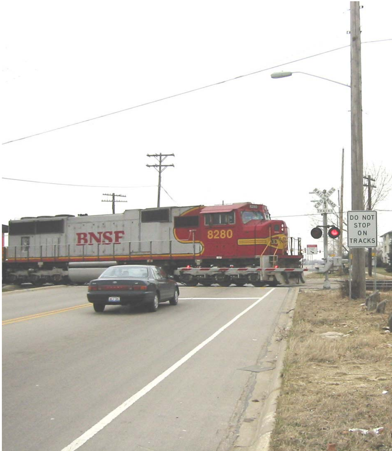
A modern freight locomotive leading a train across a two-lane rural highway-rail grade crossing. The lights and gates have been fully activated.
