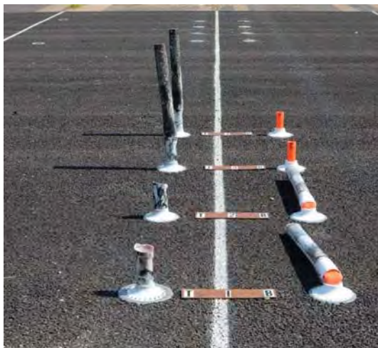
Figure 3.5. 607531-02-1 Delineators and Test Vehicle after Testing.
