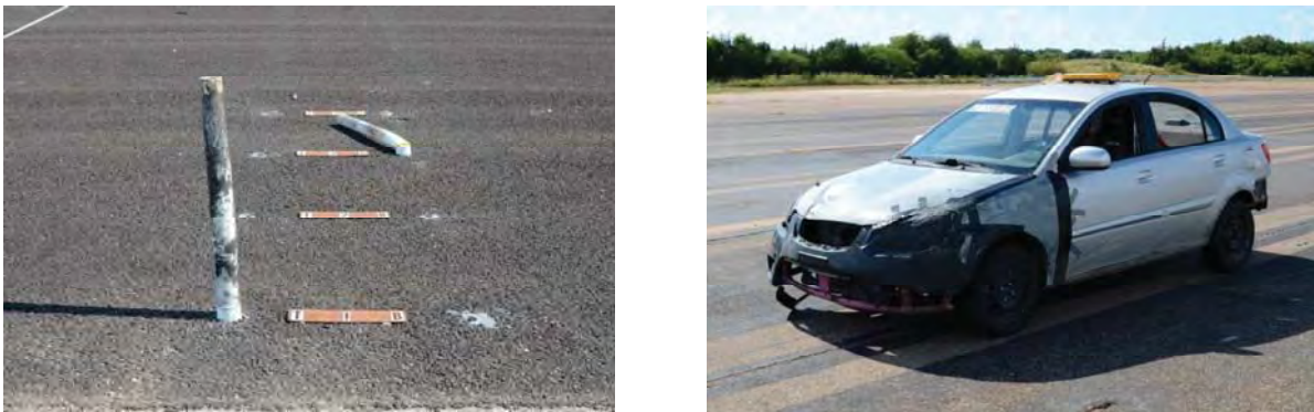
Figure 3.13. 607531-02-3 Delineators and Test Vehicle after Testing.
