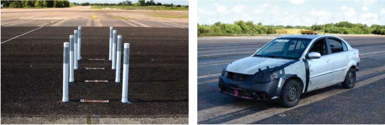
Figure 3.12. 607531-02-3 Delineators and Test Vehicle before Testing.
