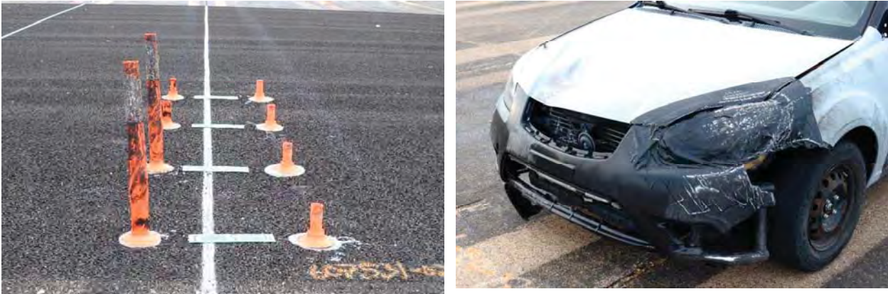
Figure 3.20. 607531-02-4 Delineators and Test Vehicle after Testing (Asphalt Surface).
