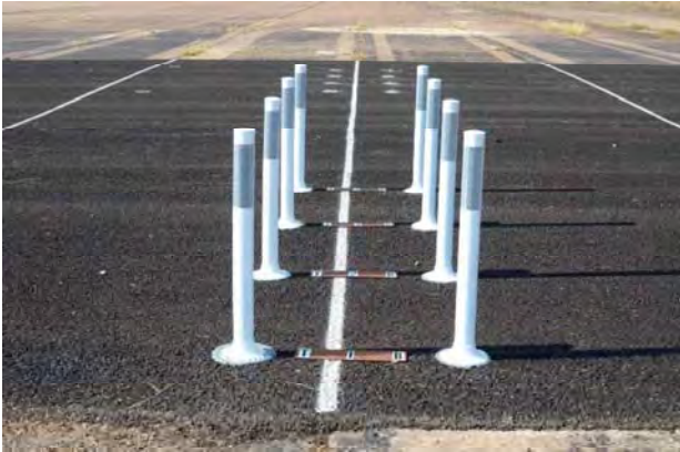
Figure 3.4. 607531-02-1 Delineators and Test Vehicle before Testing.
