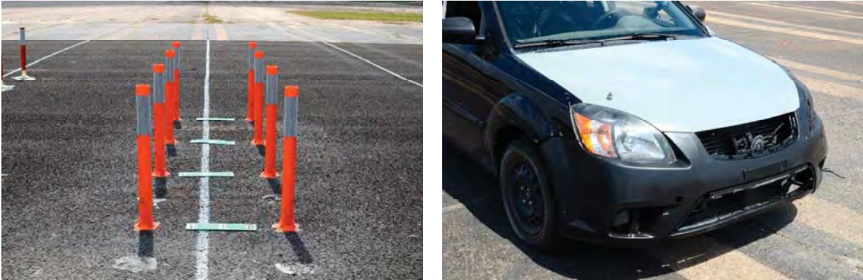
Figure 3.8. 607531-2 Delineators and Test Vehicle before Testing.
