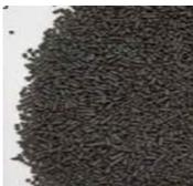
The Carbon molecular sieve used in the NGP+ has been selected for maximum performance. It has been packed to a high density and kept compact by spring loading.
