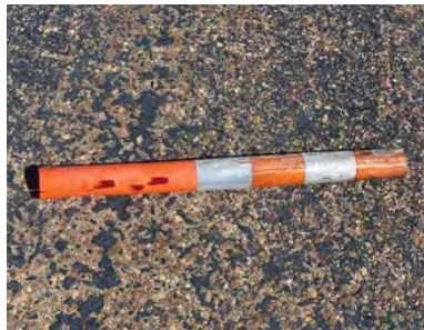
Figure A-6. Sample 3B Failure at 28 Impacts.
