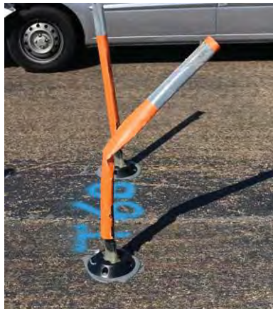
Figure A-11. Sample 6T Failure at 25 Impacts.
