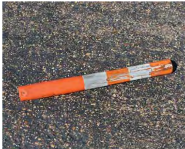
Figure A-2. Sample 1B Failure at 27 Impacts.
