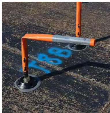
Figure A-15. Sample 8T Failure at 6 Impacts.
