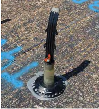
Figure A-7. Sample 4T Failure at 56 Impacts.
