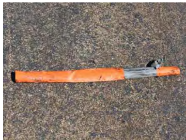
Figure A-12. Sample 6B Failure at 29 Impacts.
