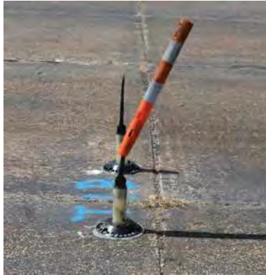
Figure A-1. Sample 1T Failure at 53 Impacts.
