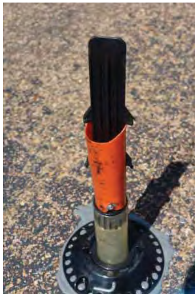
Figure A-8. Sample 4B Failure at 42 Impacts.
