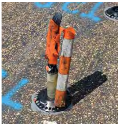
Figure A-5. Sample 3T Failure at 71 Impacts.
