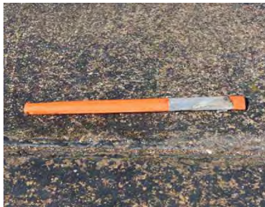
Figure A-16. Sample 8B Failure at 28 Impacts.
