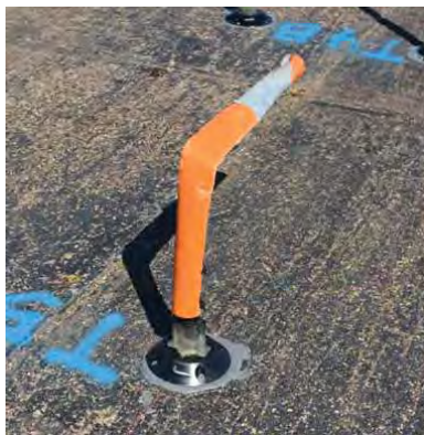
Figure A-9. Sample 5T Failure at 32 Impacts.
