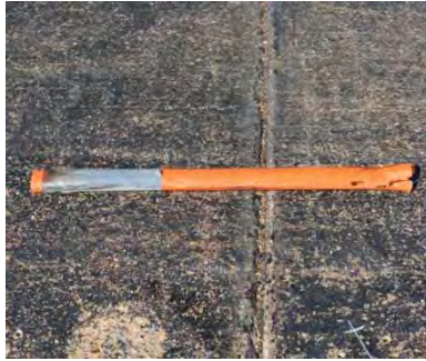
Figure A-10. Sample 5B Failure at 21 Impacts.
