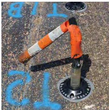
Figure A-3. Sample 2T Failure at 66 Impacts.
