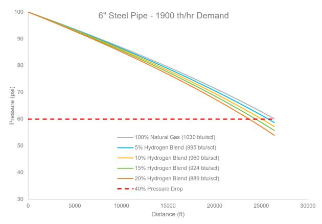
Figure 8.15: Hydrogen Blending Pressure Drop
