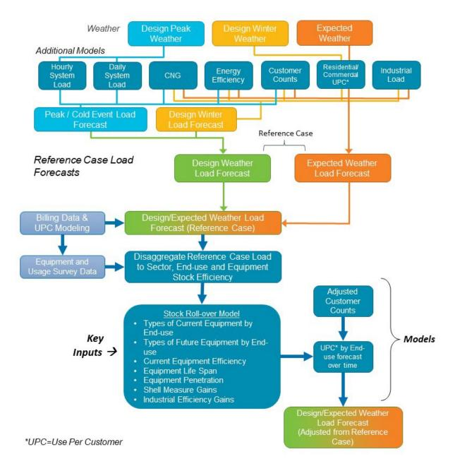
Figure 3.1: Load Forecast Model Flow Diagram
