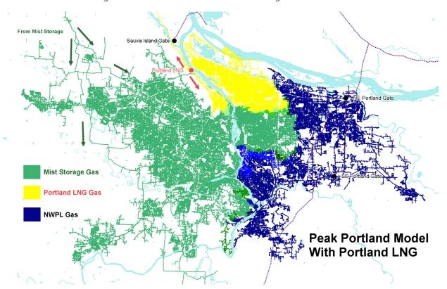
Figure 6.33: Portland LNG Gas Flow Diagram With LNG
