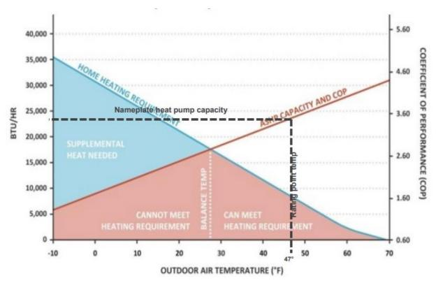
Figure 5.25: Efficiency of Electric Heat Pumps and Ambient Temperature
