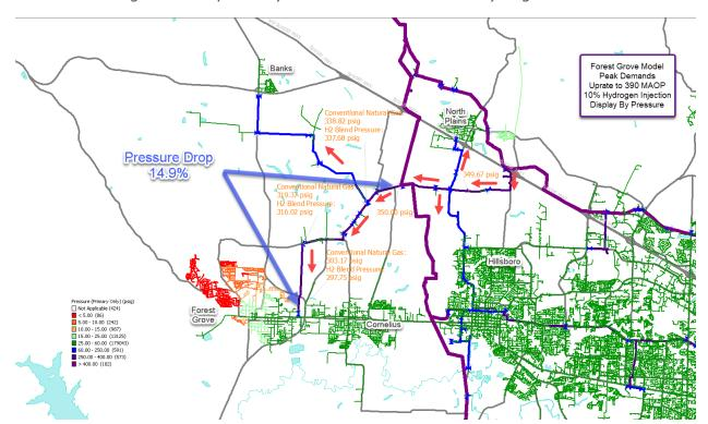
Figure 8.26: Uprated System Peak Model with 10% Hydrogen Blend
