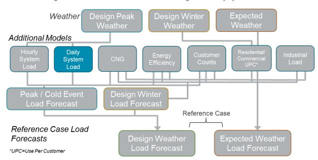
Figure 3.25: Load Forecast Model Flow Diagram – Daily System Load
