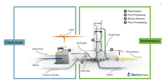
Figure 6.7: Synthetic Methane Production Process
