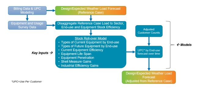
Figure 3.35: End Use Load Forecasting Process
