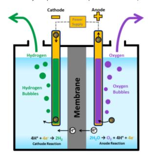
Figure 6.6: Schematic of Polymer Electrolyte Membrane (PEM) Electrolysis
