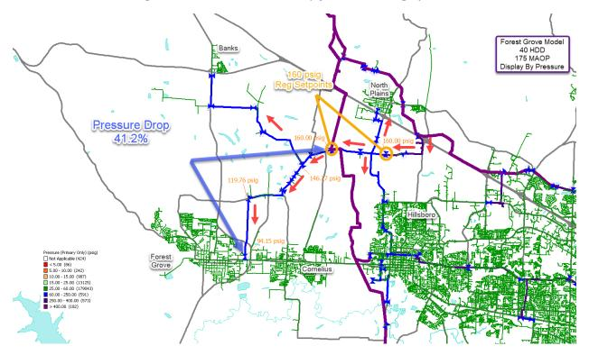
Figure 8.21: 40% Pressure Drop for the Existing System
