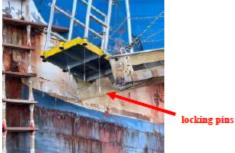
Fig. 3: Accommodation ladder with unsecured locking pins.
