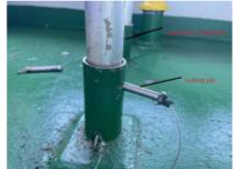
Fig. 2: Pilot boarding platform stanchion and locking pin.
