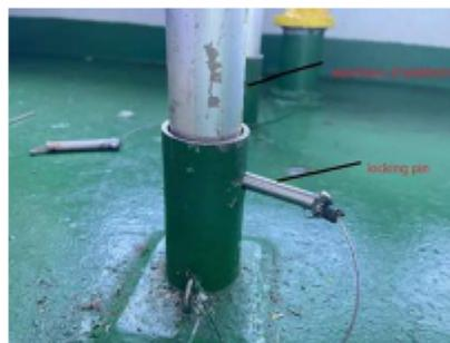
Fig. 2: Pilot boarding platform stanchion and locking pin.
