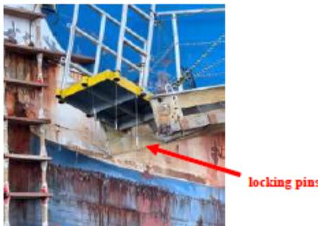
Fig. 3: Accommodation ladder with unsecured locking pins.
