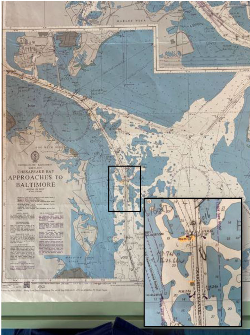
Figure 3. Paper chart that was in use and on the bridge of the EVER FORWARD at the time of the grounding. The outlined inset shows a close-up of the plotted voyage plan track line and waypoints as well as the vessel location after grounding. Photograph by USCG Investigator.
