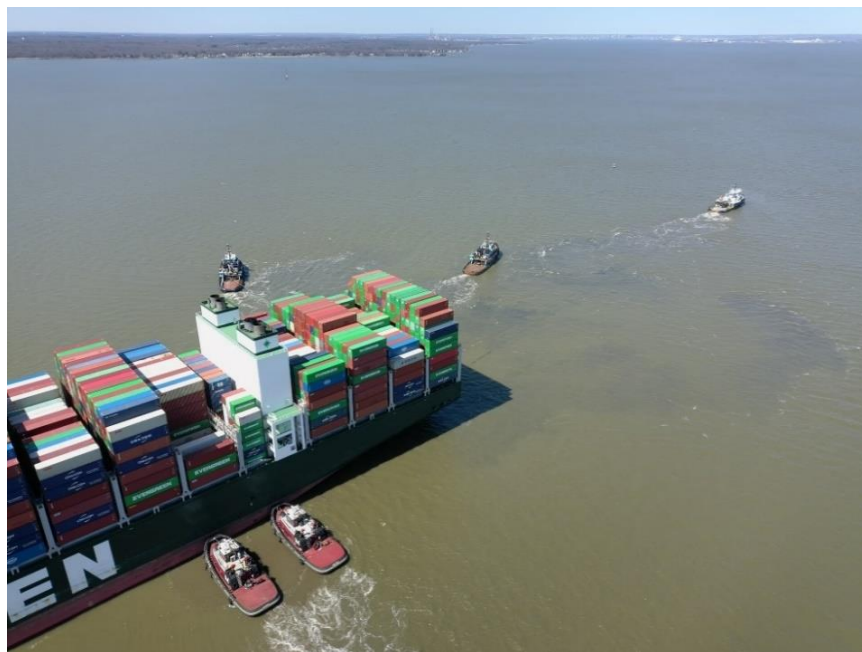
Figure 12. Aerial photo of the EVER FORWARD aft port quarter during refloat operations in an attempt to free the vessel. This photograph was provided by USCG District 5 Public Affairs.
