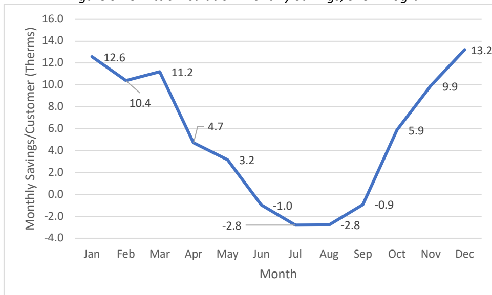
Figure 5-13: Attic Insulation Monthly Savings, Shell Program
