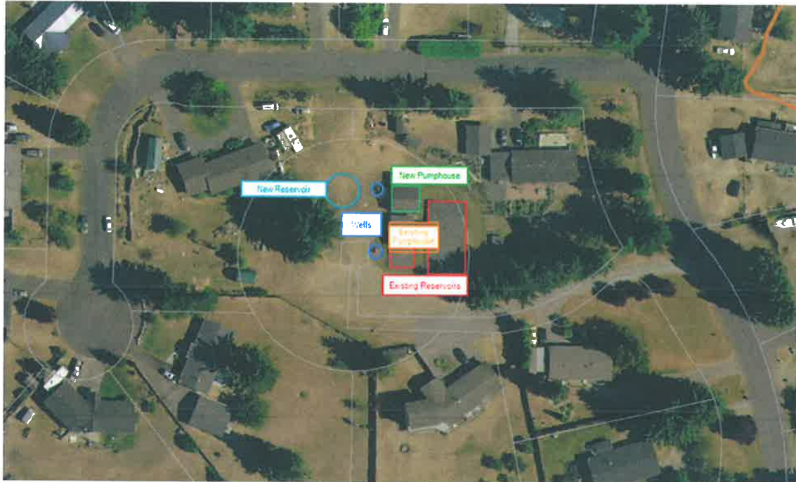
Figure 1 - Well Locations and Well Site Layout
