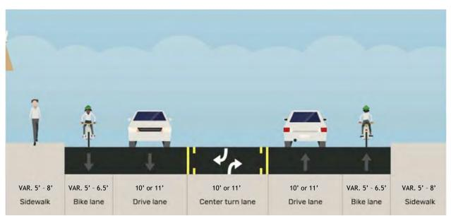
Figure 4-1. Preferred Alternative typical section.
