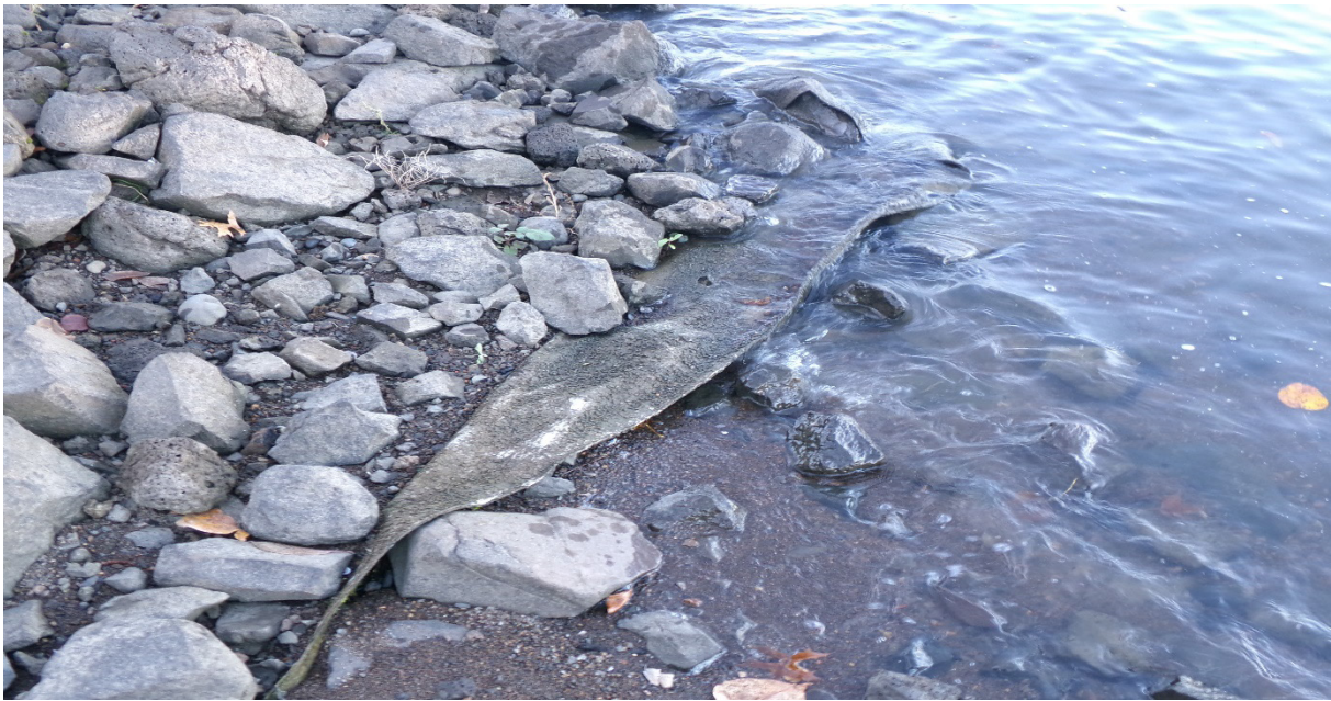
Photo 2 Organoclay Mat Material at the Midpoint of the Pilot Cap Area (11/27/2023)
