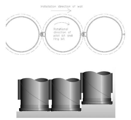
Exhibit Alt 2D-5: Principle of RD piles, interlock, and installation (Uotinen and Jokiniemi, 2012)
