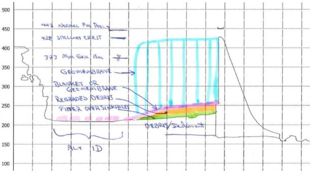
Exhibit A-Alt 1C-3: Filter over depressions and sinkholes, debris regrading, blanket, and geomembrane on slope; section perpendicular to dam
