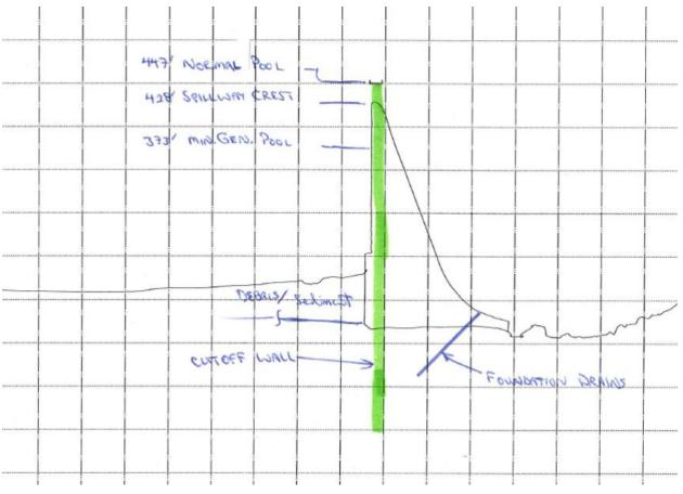
Exhibit A-Alt 2B-1: Cutoff wall through dam; section perpendicular to dam
