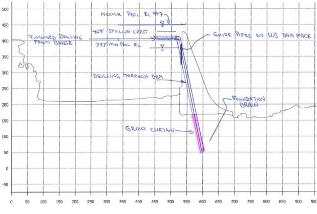
Exhibit Alt 3D-2: Grout curtain drilling from barge through upstream dam face, section perpendicular to dam
