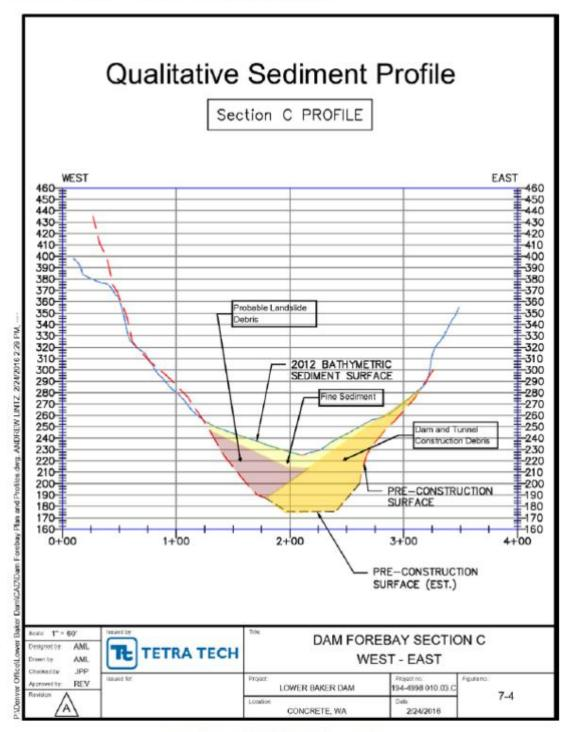
Figure 7-4: Dam Forebay Section C
