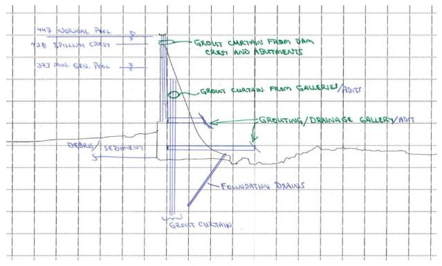
Exhibit A-Alt 3B-2: Grout curtain – drilling from adits; section perpendicular to dam
