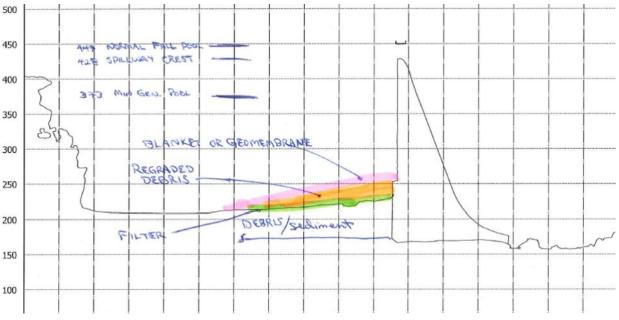
Exhibit A-Alt 1B-3: Filter over depressions and sinkholes, debris regrading, and blanket; section perpendicular to dam
