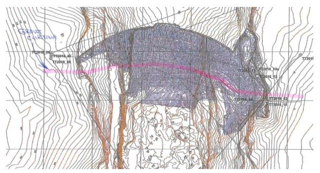
Exhibit 3E-1: Grout curtain drilling through dam from downstream dam face, plan view
