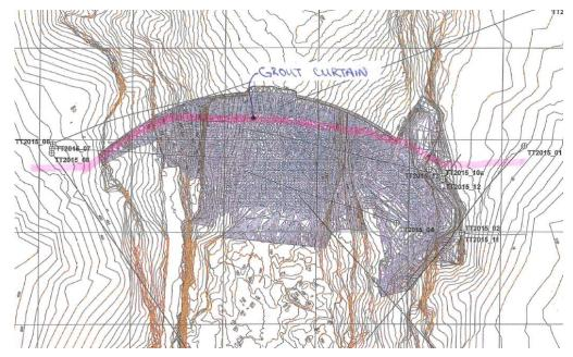
Exhibit Alt 3D-1: Grout curtain drilling from barge through upstream dam face, plan view
