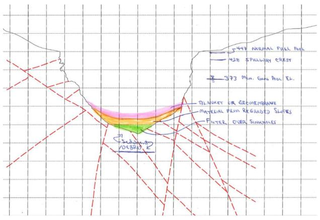
Exhibit A-Alt 1B-2: Filter over depressions and sinkholes, debris regrading, and blanket; cross section
