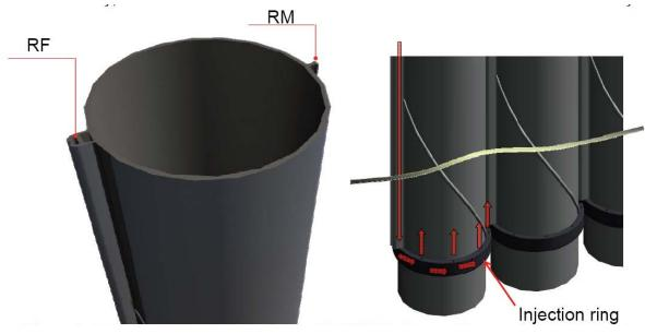
Exhibit Alt 2D-7: RD pile interlock details (left) and grout injection ring (right) (Uotinen and Jokiniemi, 2012)
