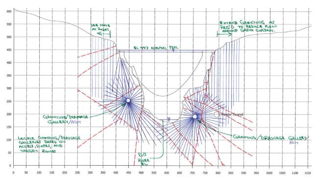
Exhibit A-Alt 3B-1: Grout curtain – drilling from adits; cross section (vertical and horizontal grout holes shown for convenience–grout hole orientations would vary and would be different on adjacent grout lines)
