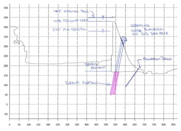
Exhibit 3E-2: Grout curtain drilling through dam from downstream dam face, section perpendicular to dam
