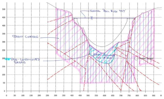
Exhibit Alt 3F-3: Grout curtain upstream of dam, drilling from barge upstream of dam, cross section (grout holes shown vertical–grout holes may be inclined and grout holes in adjacent grout curtain lines drilled at different orientations)
