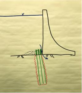
Figure 1 Potential Leakage Path
