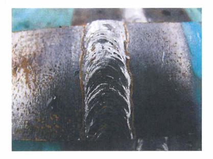
Typical **Face Bend** surface <u>prior</u> to <u>grinding</u> the specimen as preparation for testing.
