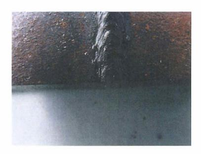
Typical **Nick Break** sample, (**end view**) prior to testing the specimens, this is to indicate the <u>depth of nick at the ends</u> of the tensile section being the preparation for testing.
