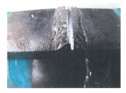
Typical **Nick Break** sample, (<u>face side</u>) prior to testing the specimens, this is to indicate the **depth of nick** along the top of the weld reinforcement or cap pass and at the ends of the tensile section.
