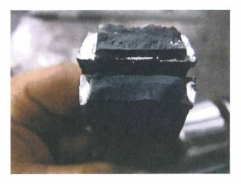
Both photo's are of the same samples turned different directions in order to fully see or evaluate the cross section. This shows the value of the nick break specimen.
