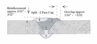
Weld Joint Design Single V-Groove
