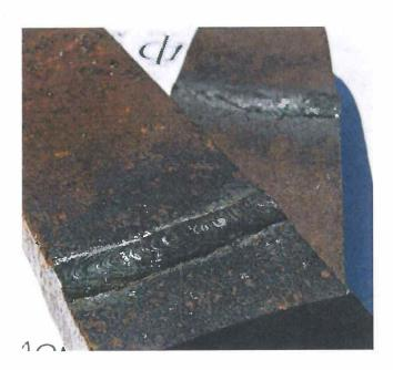
Typical **Root Bend specimens** showing the surface prior to grinding as part of the preparation for testing.
