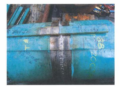
This photo shows the basic layout for the "Cutting and removal" of the required tensile specimens. Tensile specimens are removed from both <u>Sides 1 & 2</u> as shown by the <u>single</u> and <u>double lines</u> across the specimens.
