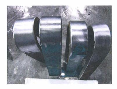
Normal set of Root and Face Bends. "Green" side specimens are Face Bends -OD of Pipe. "Brown" side specimens are Root Bends—ID or pipe.
