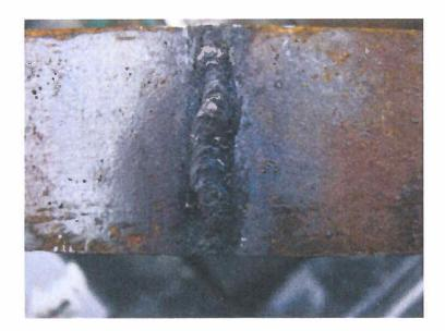
Typical **Root Bend** surface prior to grinding the specimen as preparation for testing.
