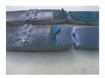
This set of **Tensile Specimens** being viewed from the side of the pipe, provides a realistic view showing the distance from the weld fusion line or toe of the weld face to the region at which the specimen failed. This is a reasonable and normal condition to expect when performing the weld tensile testing with the reinforcement remaining on the pipe specimens.
