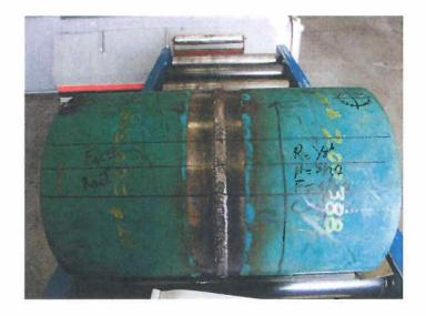
This photo shows or represents the basic layout for the "Order of removal" and <u>locations</u> for the required specimens.
