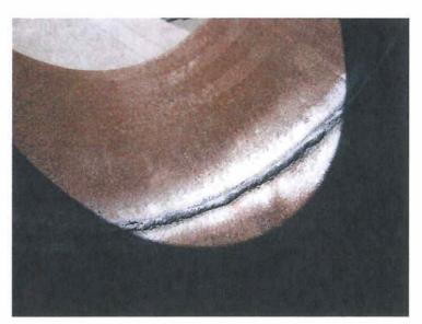
Side I - is welded using 1/8" diameter electrodes for the <u>root pass</u>.
