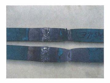
Normal set of **Tensile Specimens** being viewed from the OD or top face of the pipe. Notation should be given as to where the specimens actually necked down (reduced in cross section) and finally broke. This implies that the weld joint or weld-ment is stronger than the base material. Secondly, that the combined effects of the reinforcement played a roll to induce the failure to occur, "outside the weld Heat Affected Zone".
