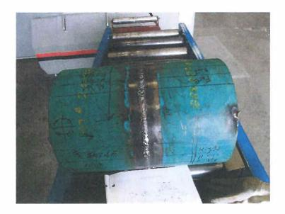
Side 2- is welded using 5/32" diameter electrodes for the root pass. The remainder of the layers, being the (a) hot pass (5/32" diameter electrodes), (b) fill and (c) cap passes are welded using 3/16" diameter electrodes.
