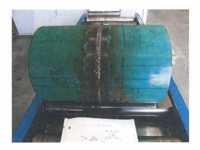
This photo shows the basic layout for the "Order of removal" and locations for the required specimens. Nick Break and Tensile tests. <u>Side 1</u>
