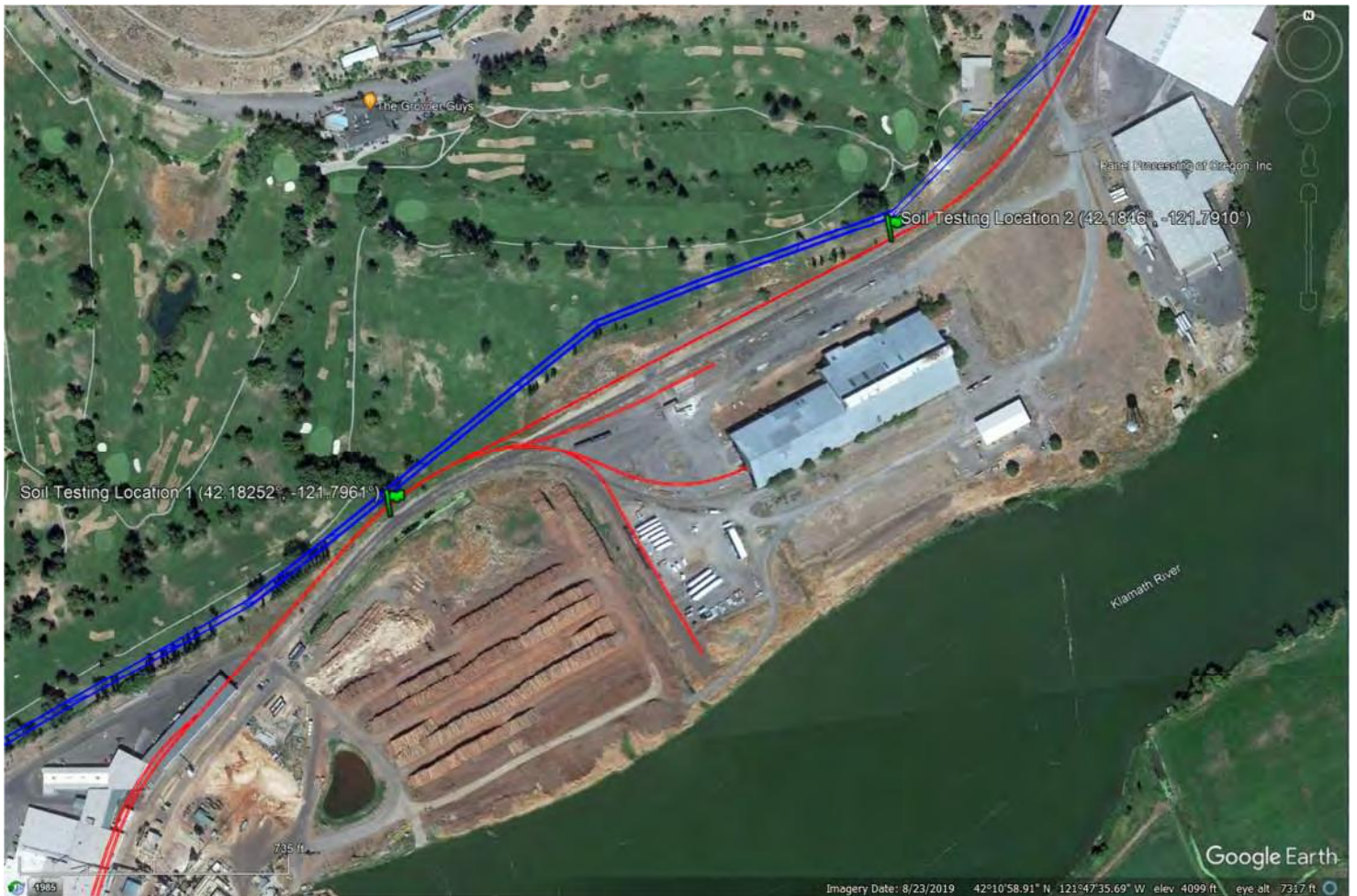
Figure 18: Soil Resistivity Measurement Locations Along Shared Corridor
