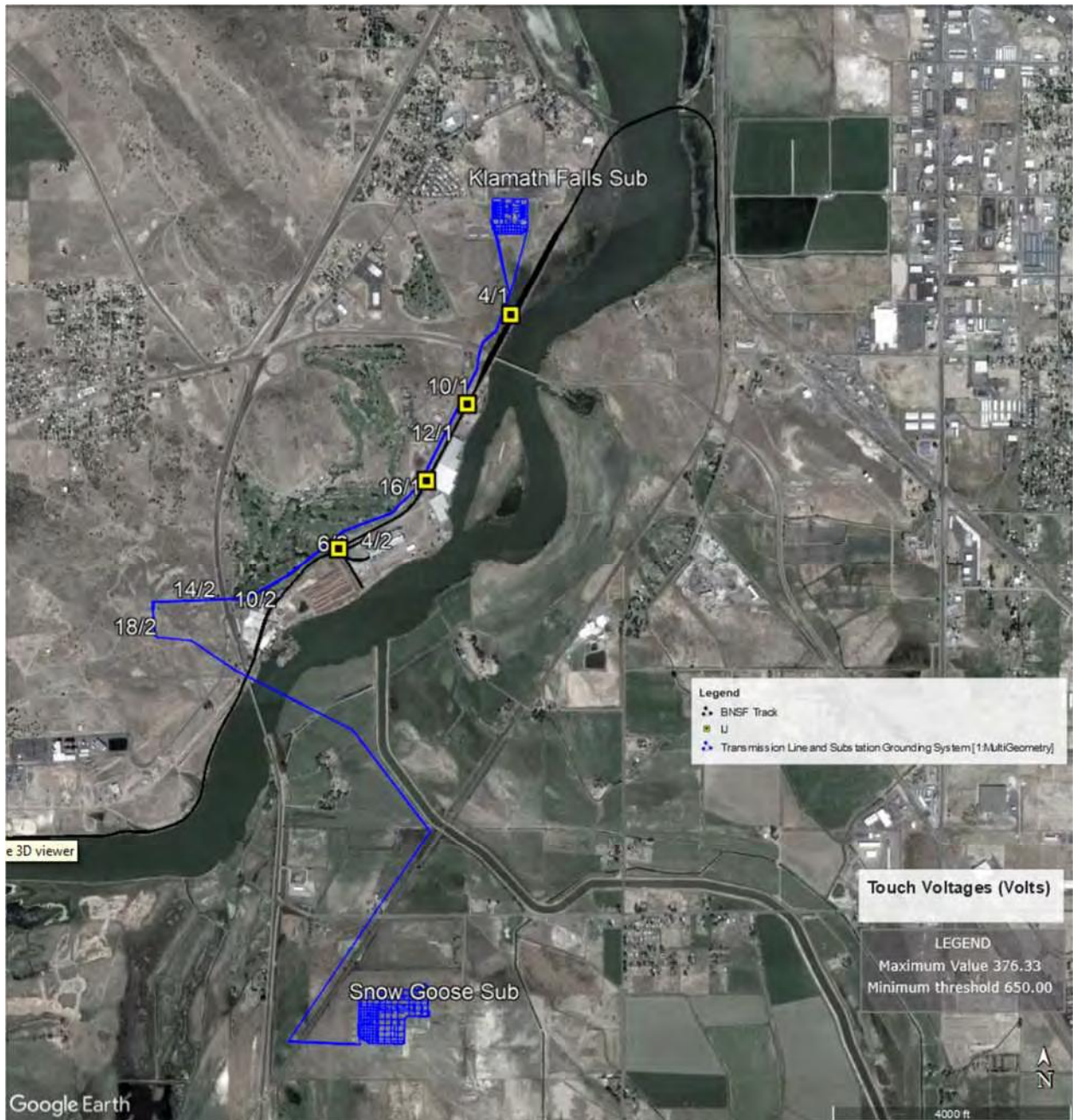
Figure 39: Mitigated Rail Touch Voltages - Faulted 230 kV Structure 6/1 - Future with 230 kV Configuration
