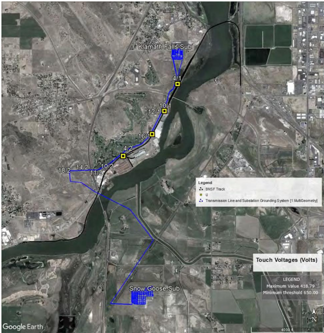
Figure 37: Mitigated Rail Touch Voltages - Faulted 69 kV Structure 9/1 - Future with 230 kV Configuration
