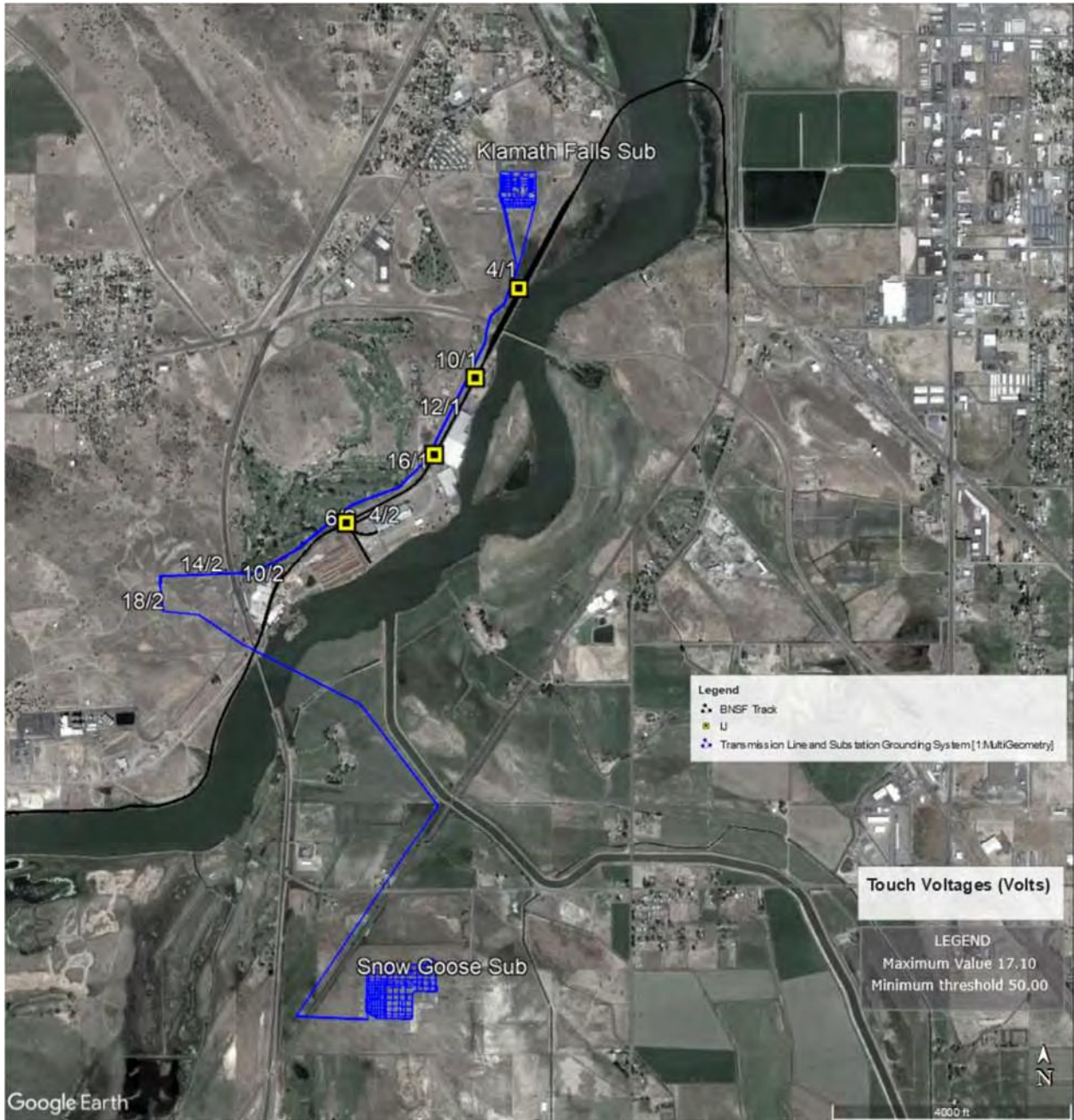
Figure 26: Rail Touch Voltages - Steady State - Future with 230 kV Configuration
