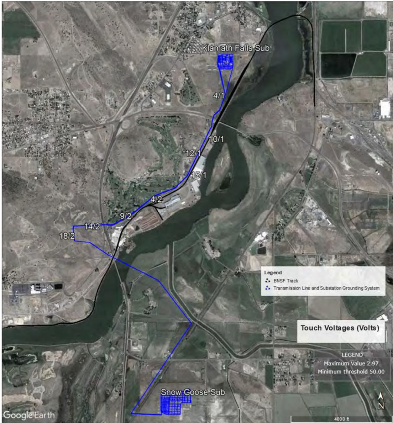
Figure 25: Rail Touch Voltages - Steady State - Existing 69 kV Configuration
