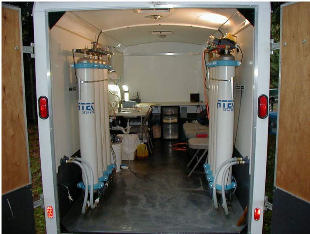
Picture above shows the interior of the pilot plant trailer from the rear. The sample outlets and the analytical equipment are on the desk in the front of the trailer.
